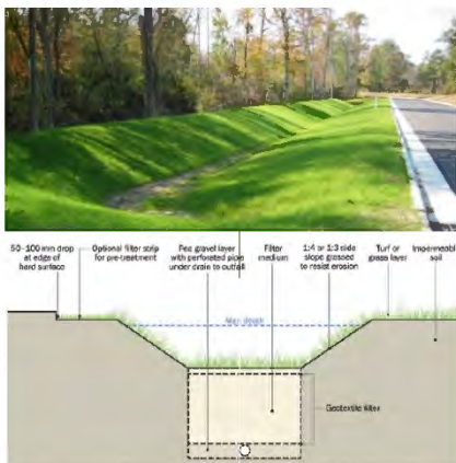
Figure 17.2 Typical dry swale
