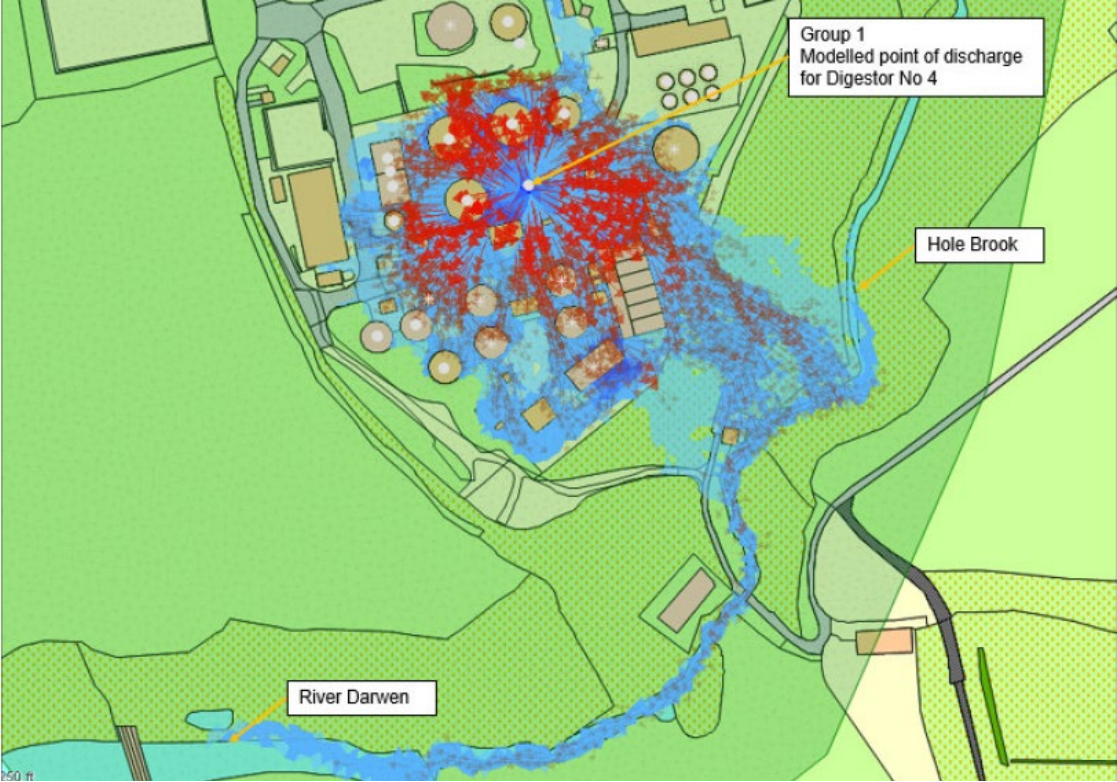
Figure 3 – Digester No. 4 Burst
