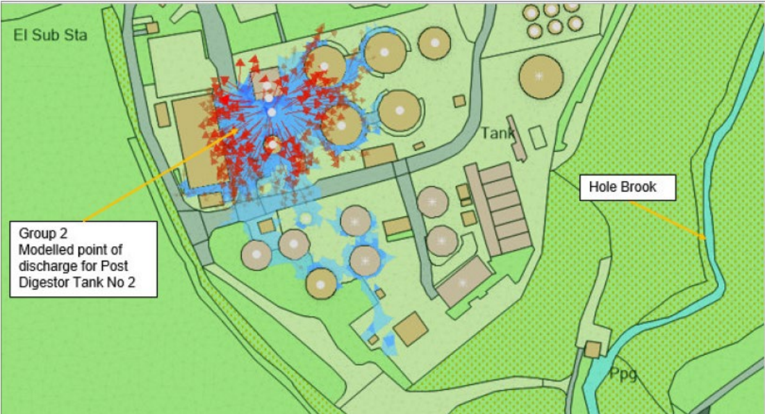
Figure 4 – Post Digestion Tank No. 2 Burst
