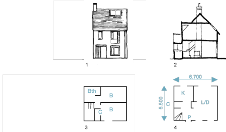
1. Front elevation 2. Section 3. First-floor 4. Ground-floor
