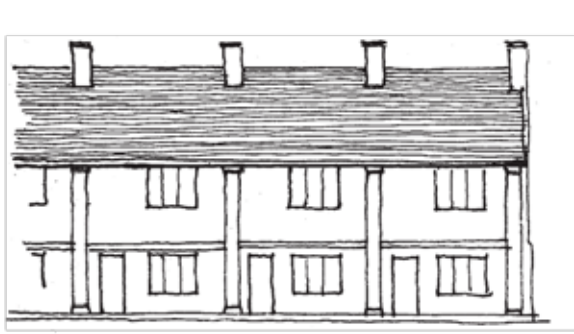
Front elevation with larger openings and facade subdivided to emphasise individual houses
