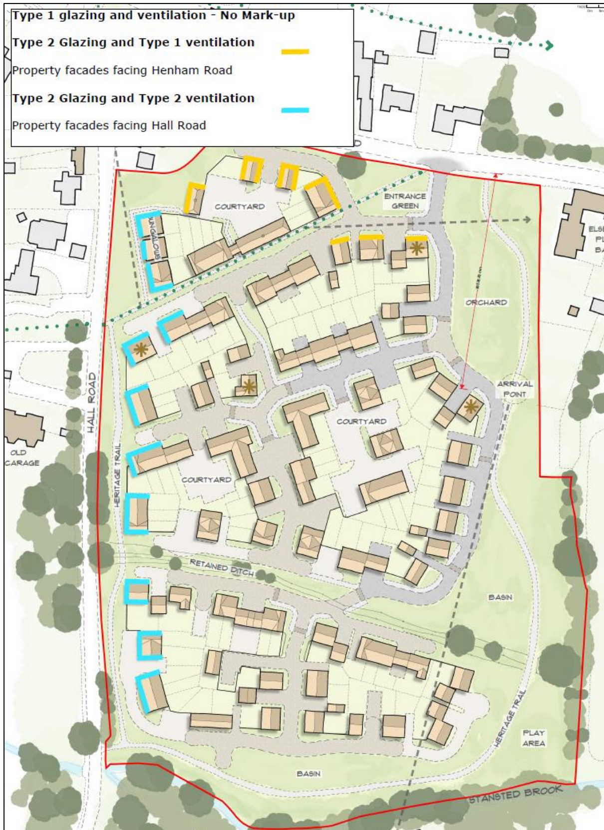
Figure 12: Facades requiring upgraded glazing and ventilation specification
