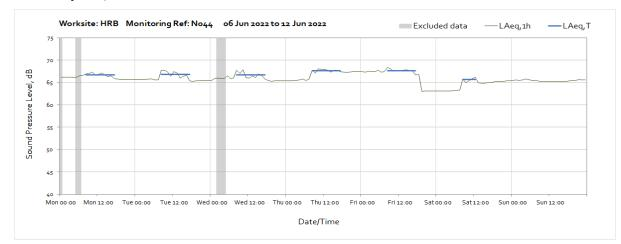
Note: The flattening of noise curve from the start of the month until 07:00 on Monday 27<sup>th</sup> June was due to additional generator fans installed close to the noise monitor. The fans were relocated into the enclosure on Monday 27<sup>th</sup> June.
