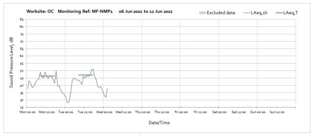
Note: Missing data from 04:00 on Wednesday 8<sup>th</sup> June were due to microphone failure. The monitor has been temporarily retrieved on Wednesday 22<sup>nd</sup> June sue to fix the microphone issue.
