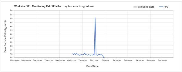
Note: Missing data from the beginning of the month till 13:00 on Wednesday 29<sup>th</sup> June was due to monitor failure caused by water ingress. Missing data from 22:00 to 23:00 on Thursday 30<sup>th</sup> June was due to a system glitch.
