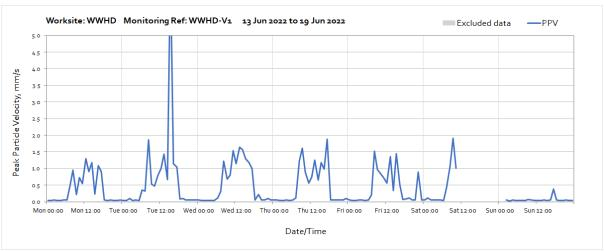
Note: High vibration levels measured throughout the week were due to digging works undertaken next to the monitoring station. The nearest sensitive receptor is 30m further away compared to the monitor and therefore HS2 vibration levels will be lower at the receptor. Missing data between 11:00 on Saturday 18<sup>th</sup> June and 01:00 on Sunday 19<sup>th</sup> June were due to a monitor's hardware error, the monitor has been reset and it's operating accordingly.
