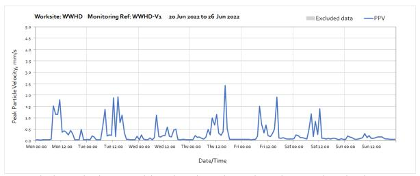
Note: High vibration levels measured throughout the week were due to digging works undertaken next to the monitoring station. The nearest sensitive receptor is 30m further away compared to the monitor and therefore HS2 vibration levels will be lower at the receptor.
