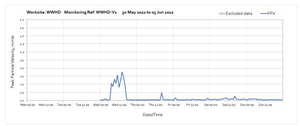
Note: High vibration levels measured between 09:00 and 15:00 on Wednesday 1<sup>st</sup> June were due to digging works undertaken next to the monitoring station. The nearest sensitive receptor is 30m further away compared to the monitor and therefore HS2 vibration levels will be lower at the receptor.
