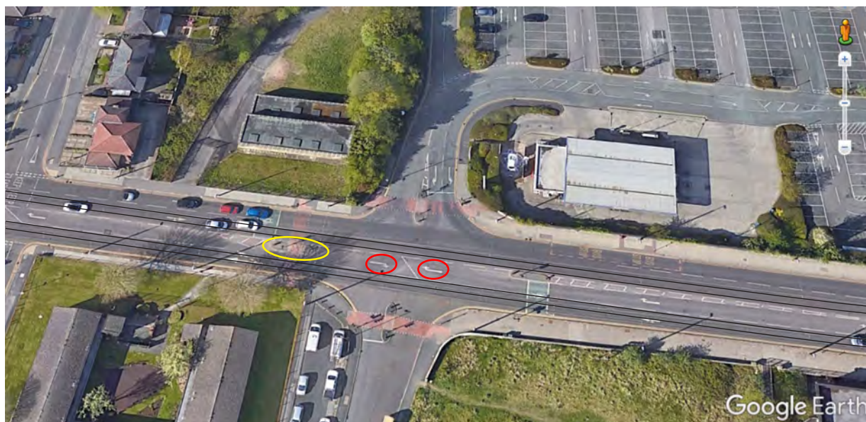
Figure 9: Right turn lanes (highlighted red) positioned between tramway tracks, with pedestrian refuge (highlighted yellow) positioned in the centre of the carriageway
