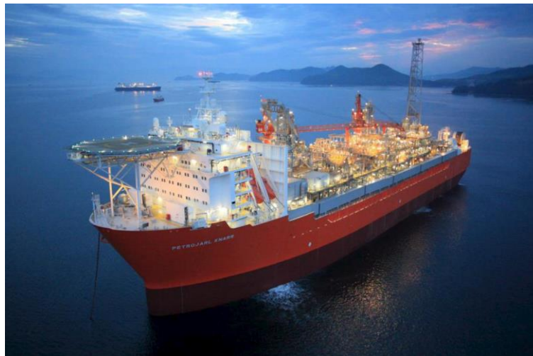
Figure 3-14 The ship-shaped FPSO which will be redeployed at Rosebank
