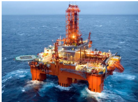
Figure 3-6 Example semi-submersible drilling rig (Source: Seadrill)
