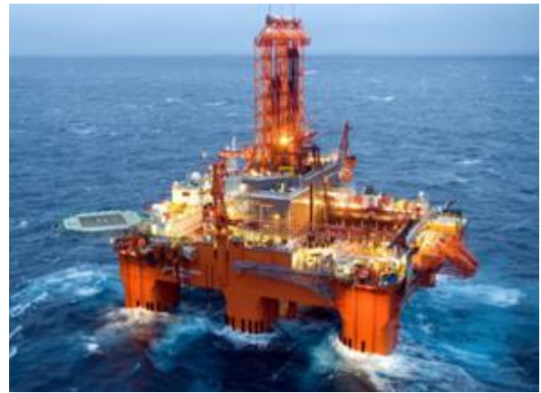
Figure 2 Example of a Semi-submersible Drilling Rig
