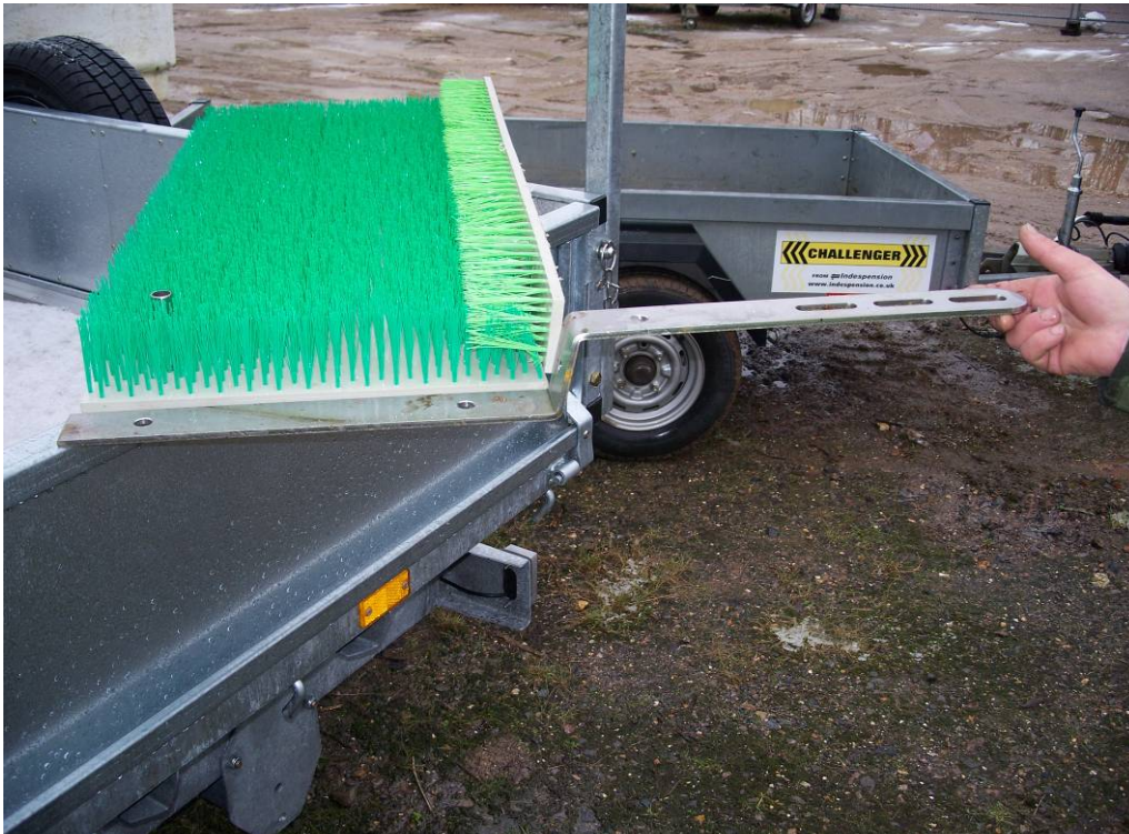
Figure 4.9: Pre-fabricated stainless steel bracket (showing stand-off)
