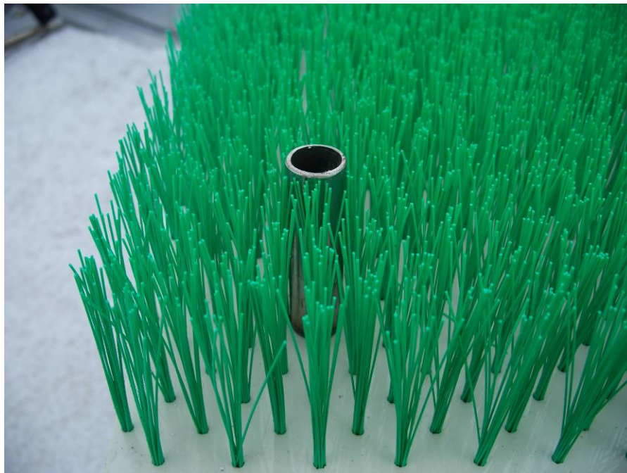
Figure 4.8: Bristle board with stainless steel spacer / nut
