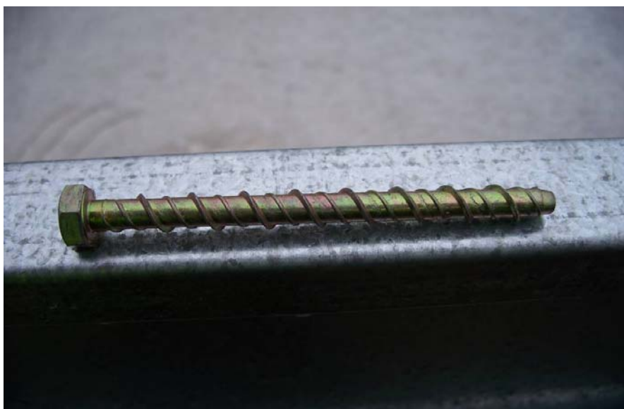
Figure 4.11: The ‘thunderbolt’ – an 8mm, self-tapping masonry bolt used to fix brackets to the wingwalls
