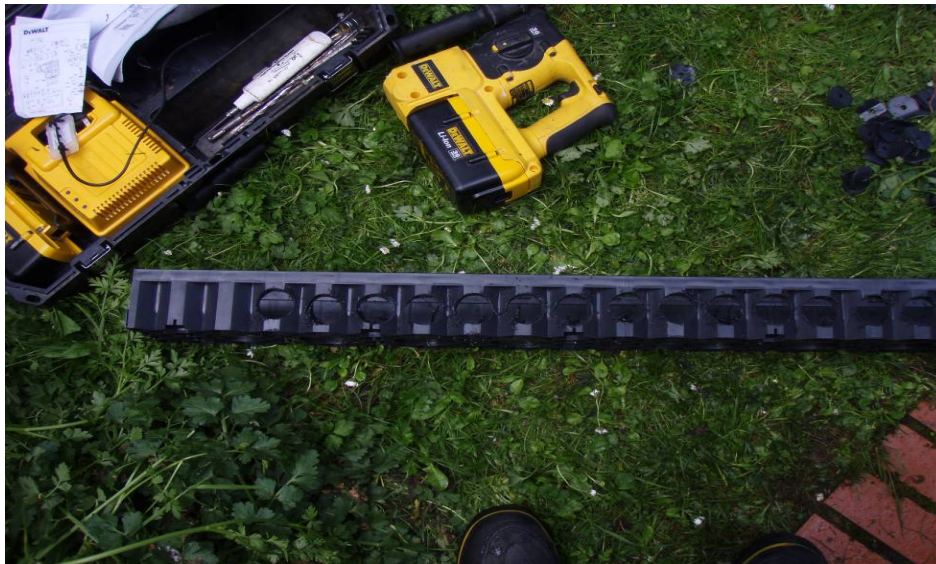
Figure 4.17: UPVC sectional channel
