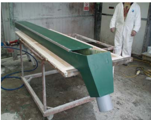
Channel with flow-splitter attached
