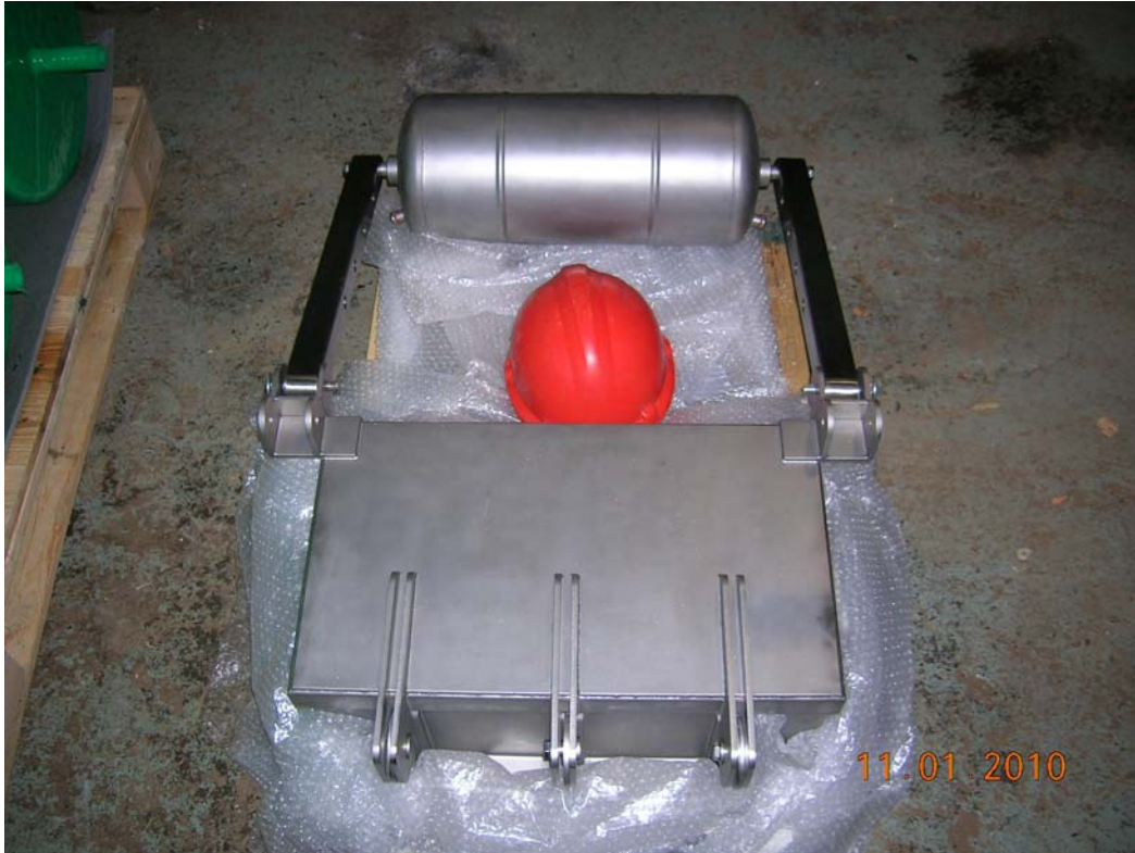
Figure 7.12: Bottom-hinged cat flap, to be installed in the tidal flap in the River Stiffkey. The door is in the closed position, with the float in the high-tide position. The dimensions of the opening are 600 x 300 mm. Photograph shown with permission of Sandy Cowie.
