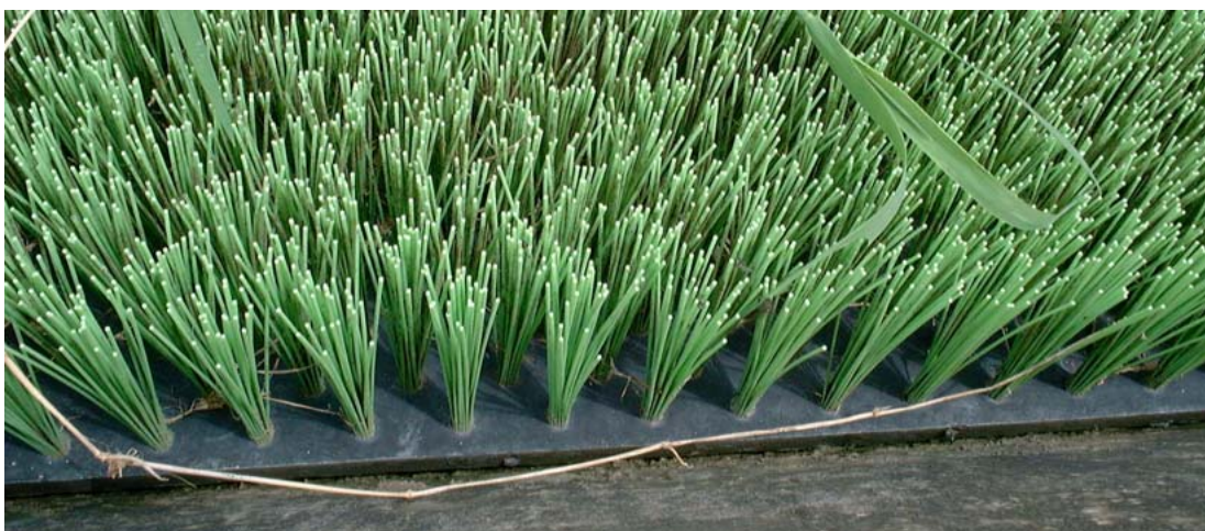
Figure 3.1: Bristle substrate with nylon bristles fixed to a polypropylene sheet
