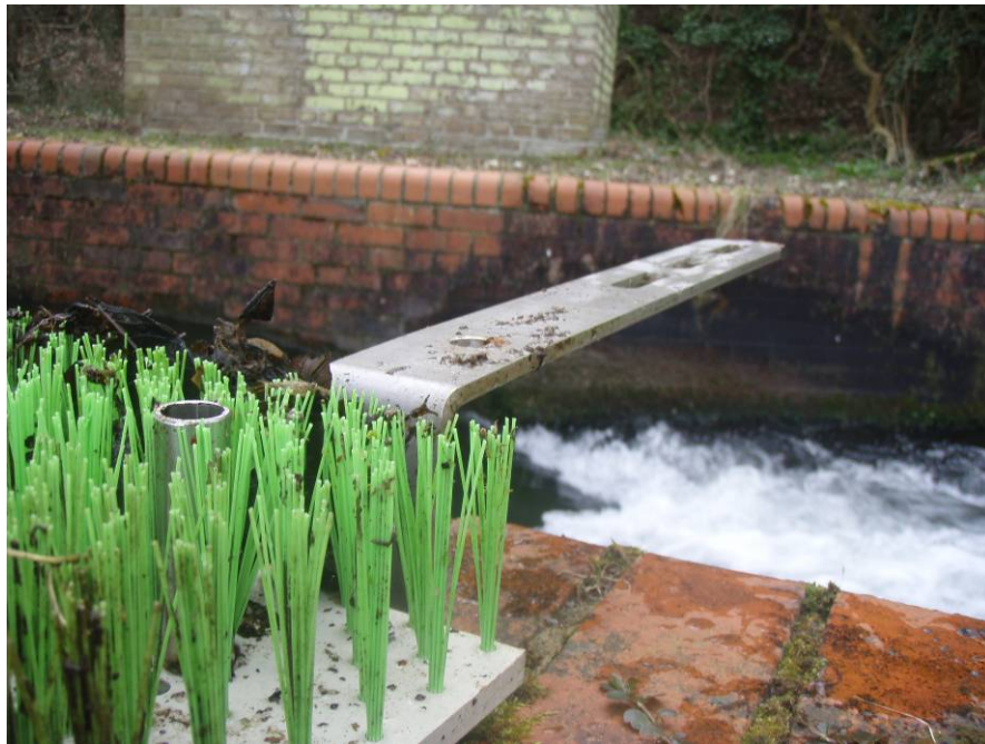
Figure 4.7: Stand-off bracket and spacer with board fixed
