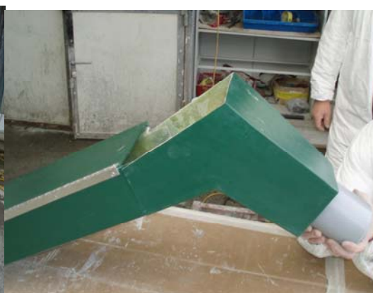
Channel with flow-splitter attached
