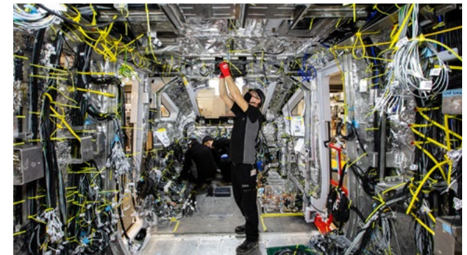
Fitting out the inside of a train in the Hitachi factory where some of the HS2 trains will be manufactured.
