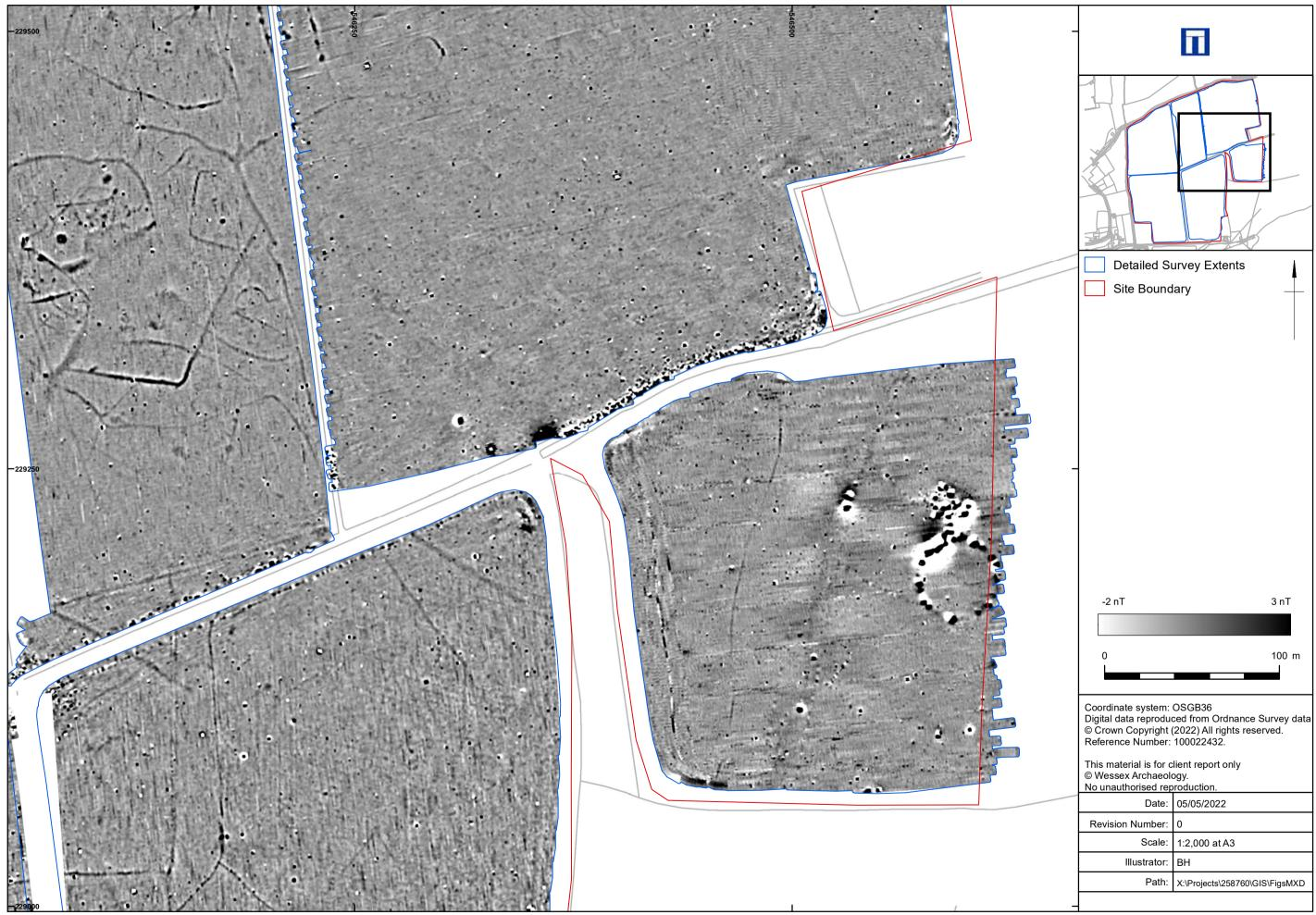
Detailed gradiometer survey results: greyscale plot (east)
