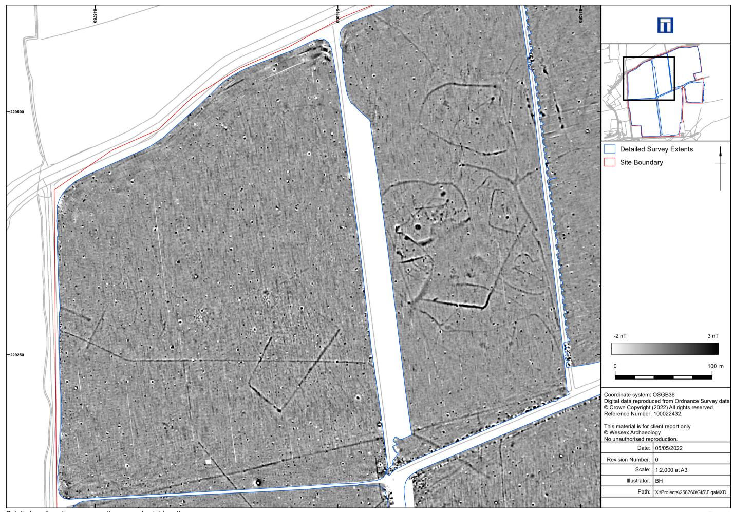
Detailed gradiometer survey results: greyscale plot (west)
