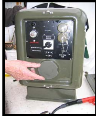
Fig 8 Air inlet blanking plate
