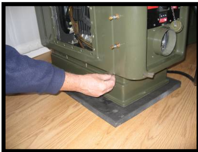
Fig 29 Casing securing clips
