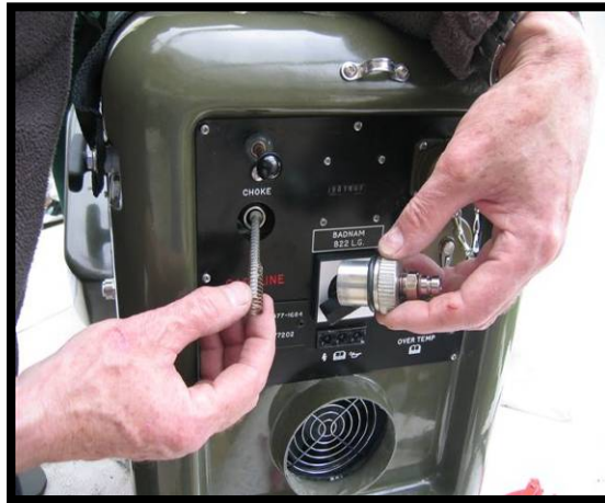
Fig 12 Front panel in line fuel filter
