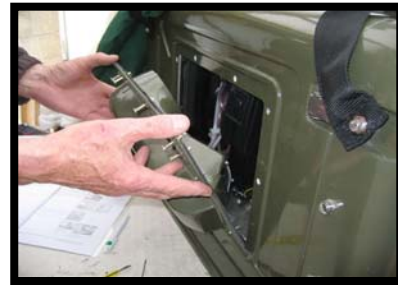
Fig 14 Engine inspection plate
