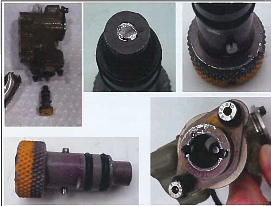
Figure 1.4.19 - Yellow MCD and MCD housing inspection.
