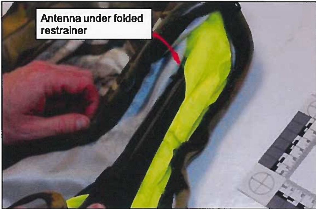
Figure 1.4.48 - Incorrect EPLB antenna positioning on a quarantined 736 NAS LSJ.
