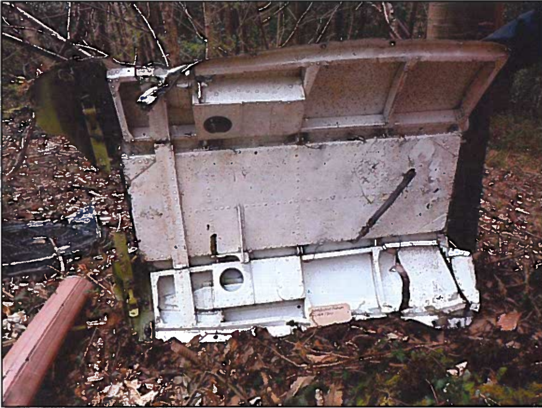
Figure 1.4.16 - Oil splatter visible on the interior of the gull wing doors.
