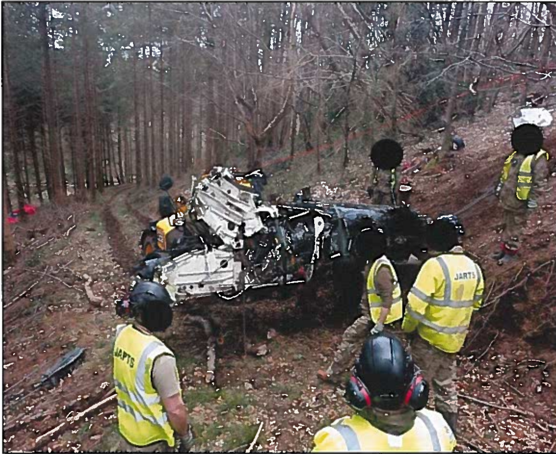
Figure 1.4.11 - Removal of the fuselage via the logging track mid-way down the slope.
