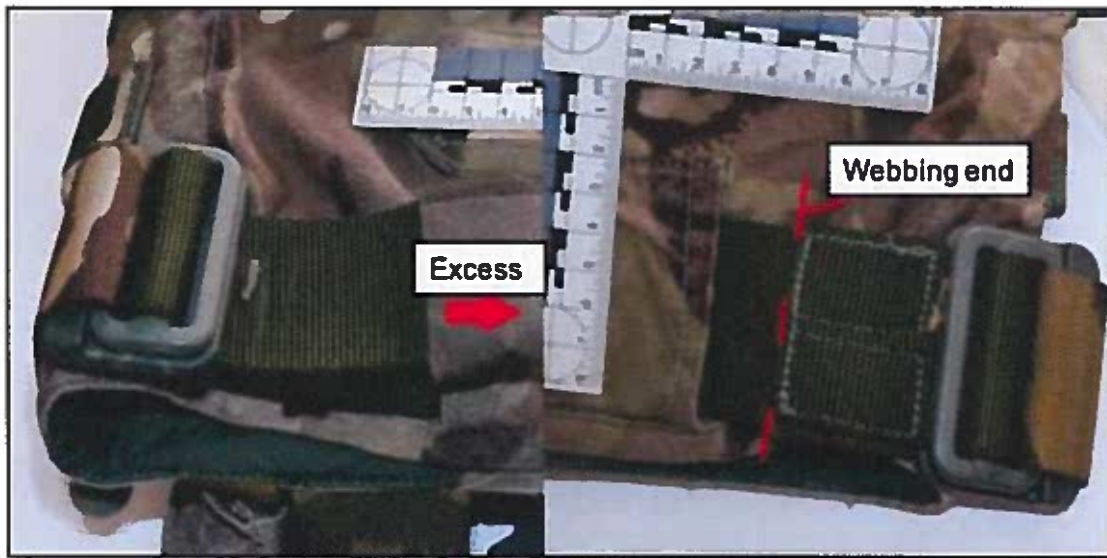
Figure 1.4.54 - Rear adjustment straps on the failed LSJ pulled asymmetrically.
