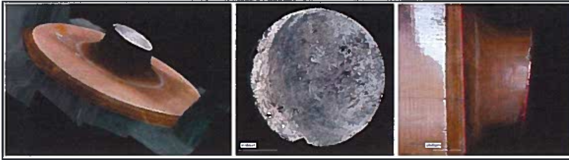
Figure 1.4.25 – Wear to the end face of the plunger from contact with the MCD.
