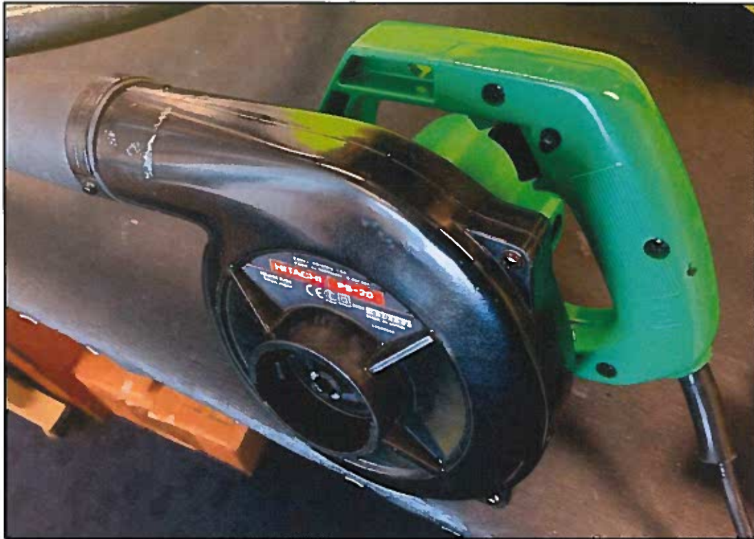
Figure 1.4.45 - Incorrect Inflator / Deflator used by 736 NAS for LSJ inflation tests.
