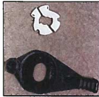
Figure 1.4.59 - Visor locking cam.
