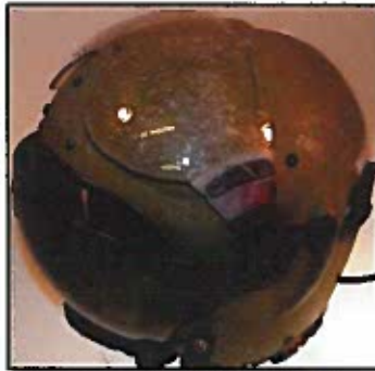
Figure 1.4.58 - MDC visor spatter.
