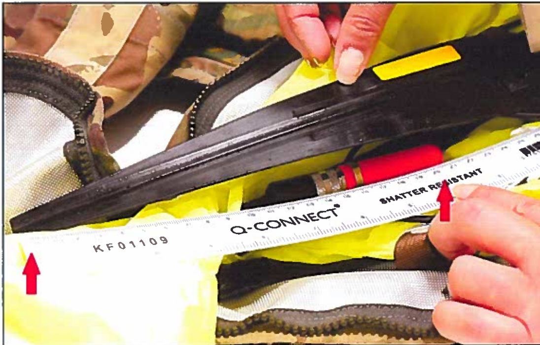
Figure 1.4.44 - Position measurements for the EPLB antenna on a reference LSJ.
