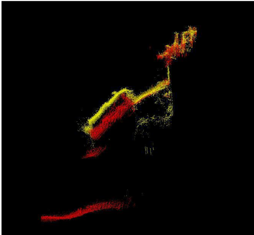
Figure 21 – Longitudinal cross-section showing area of continued change (yellow: 2020 survey, red: 2021 survey)
