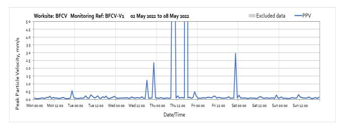
Note: High PPV level was due to a local disturbance to the vibration monitor.
