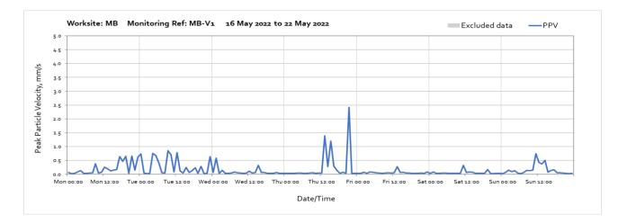
Note: High vibration levels measured throughout the week were due to local disturbance of the monitor and are not representative of HS2 vibration levels at the receptor.
