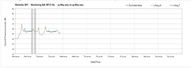
Note: Missing data between 24/05/2022 at 22:00 pm and 31/05/2022 at 23:00 pm due to a power disconnection.
