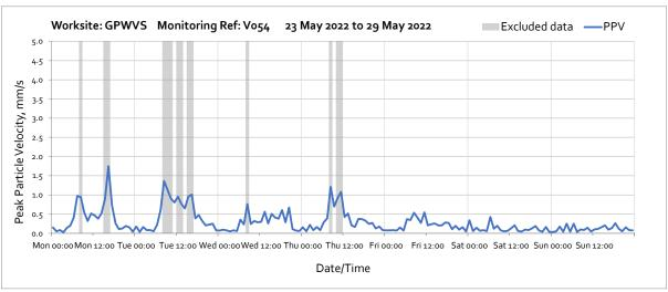
Note: High vibration levels measured throughout the week were due to local disturbance at the monitoring location and not representative of HS2 vibration levels at the receptor.
