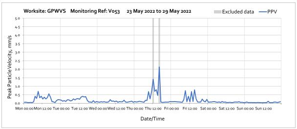
Note: High vibration levels measured at 12:00 and 16:00 on Thursday 26<sup>th</sup> May were due to local disturbance at the monitoring location and not representative of HS2 vibration levels at the receptor.
