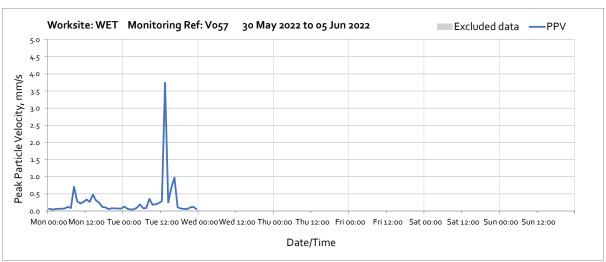
Note: High vibration levels measured at 13:00 and 16:00 on Tuesday 31<sup>st</sup> May were due to floor sawing/breaking out works undertaken next to the monitoring station. The nearest sensitive receptor is 10m further away compared to the monitor and therefore HS2 vibration levels will be lower at the receptor.
