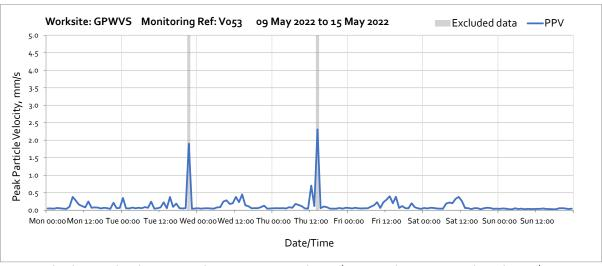
Note: High vibration levels measured at 21:00 on Tuesday 10<sup>th</sup> May and at 14:00 on Thursday 12<sup>th</sup> May were due to local disturbance at the monitoring location and not representative of HS2 vibration levels at the receptor.
