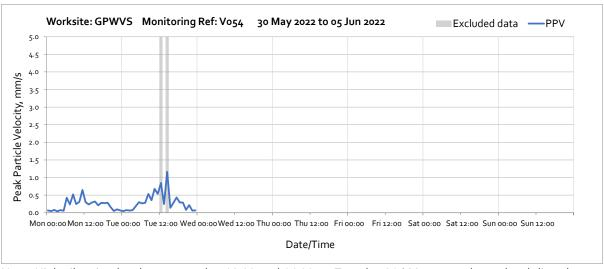
Note: High vibration levels measured at 12:00 and 14:00 on Tuesday 31<sup>st</sup> May were due to local disturbance at the monitoring location and not representative of HS2 vibration levels at the receptor.
