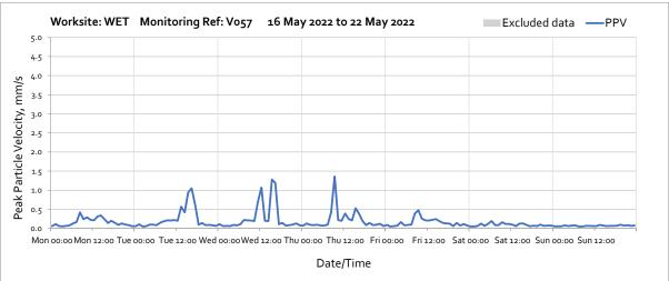
Note: High vibration levels measured during Wednesday and Thursday were due to floor sawing/breaking out works undertaken next to the monitoring station. The nearest sensitive receptor is 10m further away compared to the monitor and therefore HS2 vibration levels will be lower at the receptor
