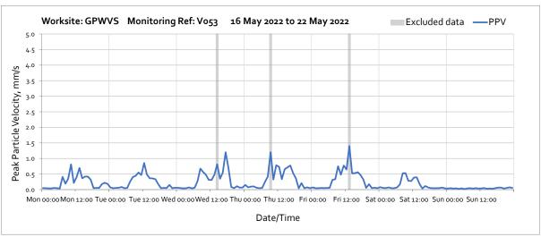
Note: High vibration levels measured throughout the week were due to local disturbance at the monitoring location and not representative of HS2 vibration levels at the receptor.
