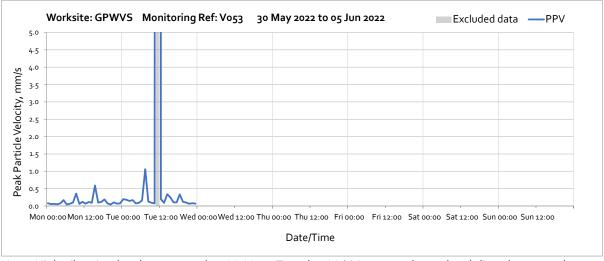
Note: High vibration levels measured at 11:00 on Tuesday 31st May were due to local disturbance at the monitoring location and not representative of HS2 vibration levels at the receptor.
