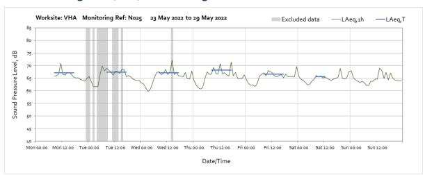
Note: Missing data from the beginning of the month to 08:00 on Monday 23<sup>rd</sup> May 2022 was due to loss of continuous power supply to the lighting column which powers the monitoring station.
