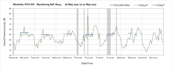
Note: Missing data between 10:00 and 11:00 on Wednesday 18<sup>th</sup> May 2022 was due to the monitoring station being switched off for routine maintenance.
