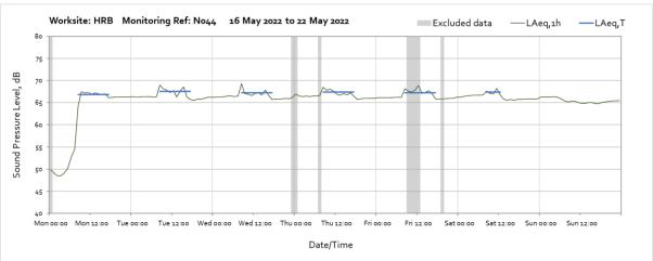
Note: The flattening of noise curve from 16<sup>th</sup> May onwards was due to additional generator fans installed close to the noise monitor.
