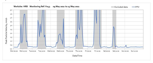
Note: High levels of vibration measured throughout the week were due to utility diversion works undertaken in proximity to the monitoring station. The monitor has had to be moved from its mounting to make way to advancing utility diversion works in the area and is therefore not firmly connected to a structure while a permanent location is being arranged with Camden Council. Due to this, readings are not representative of actual impacts.
