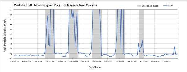
Note: High levels of vibration measured throughout the week were due to utility diversion works undertaken in proximity to the monitoring station. The monitor has had to be moved from its mounting to make way to advancing utility diversion works in the area and is therefore not firmly connected to a structure while a permanent location is being arranged with Camden Council. Due to this, readings are not representative of actual impacts.
