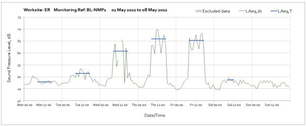
Note: Missing data at 13:00 on Wednesday 4<sup>th</sup> May were due to maintenance of the monitoring station.
