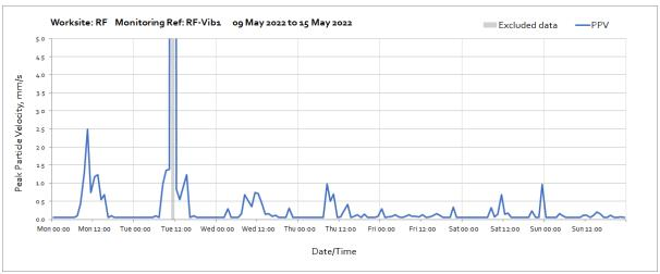
Note: High vibration level measured at 11:00 on Tuesday 10<sup>th</sup> May were due to local disturbance at the monitoring station and not representative of HS2 vibration level at the nearest receptor.
