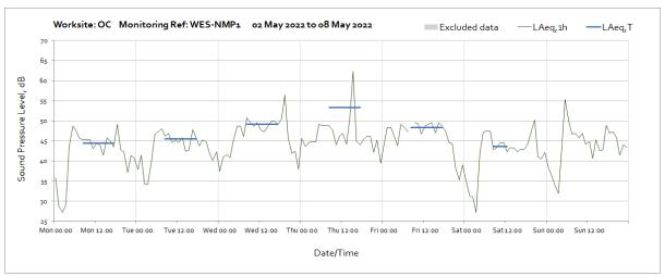
Note: Missing data at 08:00 on Friday 6st May were due to maintenance of the monitoring station.
