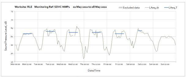
Note: Missing data at 13:00 on Wednesday 4<sup>th</sup> May were due to maintenance of the monitoring station.
