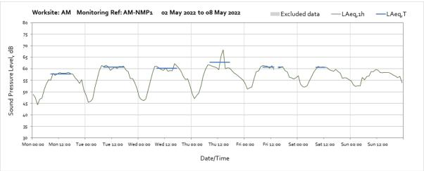
Note: Missing data between 14:00 and 15:00 on 6<sup>th</sup> May was due to monitor field calibration.
