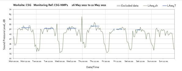
Note: Missing data between 10:00 and 11:00 on 20th May was due to monitor maintenance.
