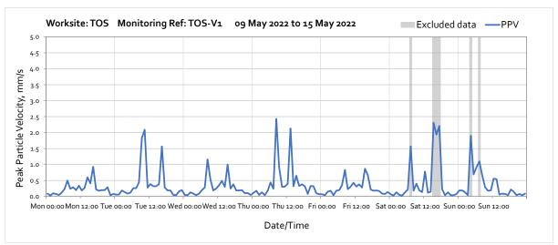
Note: High vibration levels measured throughout the weekend were due to local disturbance to the monitor station, therefore they were not representative of HS2 vibration level at the nearest sensitive receptor.
