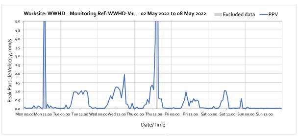
Note: High vibration levels measured at 13:00 on Monday 2<sup>nd</sup> May were due to local disturbance to the monitor station, therefore they were not representative of HS2 vibration level at the nearest sensitive receptor. High vibration levels measured at 14:00 on Thursday 5<sup>th</sup> May were due to field calibration.
