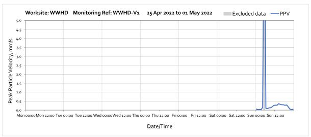
Note: High vibration levels measured at 5:00 on Sunday 1<sup>st</sup> May were due to local disturbance to the monitor station, therefore they were not representative of HS2 vibration level at the nearest sensitive receptor.
