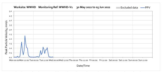
Note: High vibration levels measured throughout the week were due to digging works undertaken next to the monitoring station. The nearest sensitive receptor is 20m further away compared to the monitor and therefore HS2 vibration levels will be lower at the receptor.
