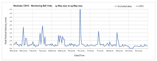
Note: High PPV measured at 11:00 on  $26^{th}$  May due to fencing works on boundary taking place in line with S61 in close proximity to monitor.
