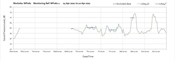
Note: Missing data on between 07:00 from  $4^{th}$  April to 15:00 on  $6^{th}$  April was due to outages caused by the equipment suffering system errors. It was manually re-set by the provider however no data recovery was possible for the outages.
