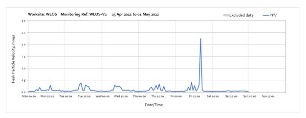
Note: High vibration levels measured during the week were due to heavy machinery passing close to the monitor.
