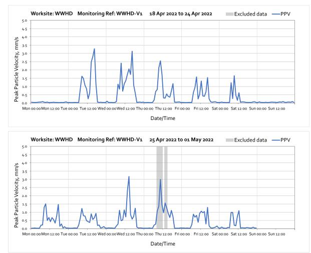
Note: High vibration levels between from 08:00 until 11:00 and from 13:00 until 14:00 on Thursday 28<sup>th</sup> April were due to local disturbance to the monitor station, therefore they were not representative of HS2 vibration level at the nearest sensitive receptor.
