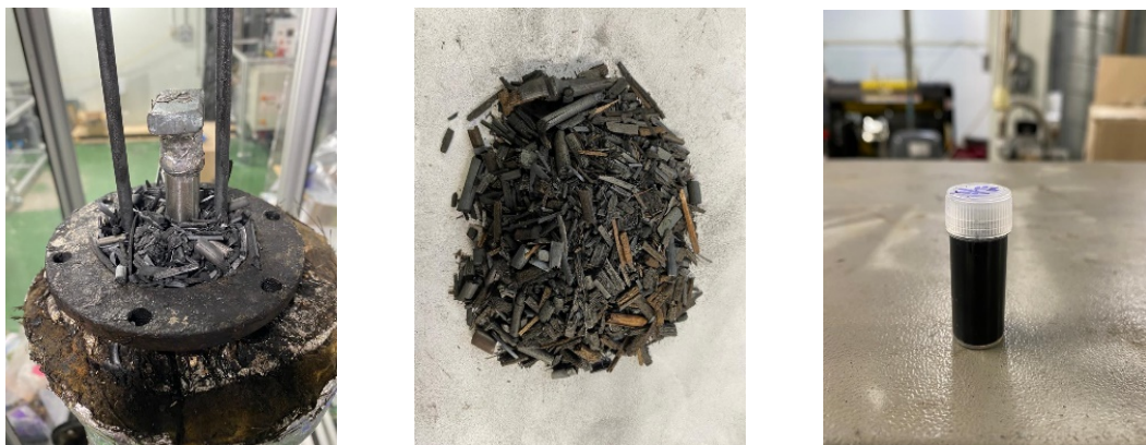
Figure 9 Torrefaction experiments showing the reactor, and torrefied and liquid products (left to right)
