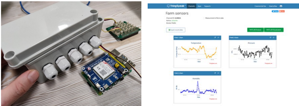
Figure 6 In-field sensors and example plots
