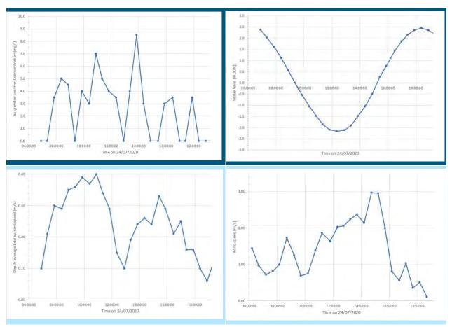
Figure 6.27 Timeseries of SSC (top left), water level (top right), current speed (bottom left) and wind speed (bottom right) during spring tide surveys on 24<sup>h</sup> July 2020
