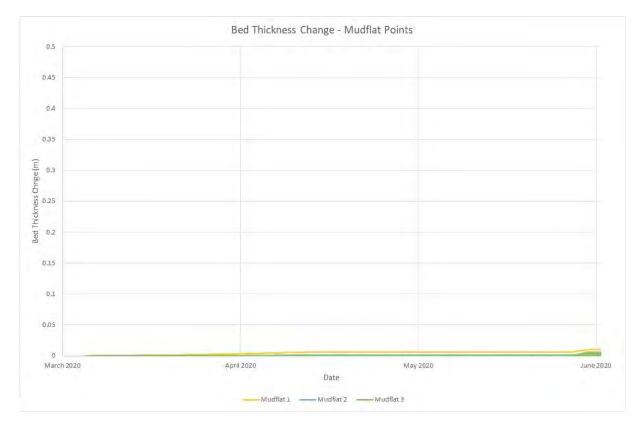
Figure 6.55 Timeseries of changes in sediment deposition at the mudflat monitoring points
