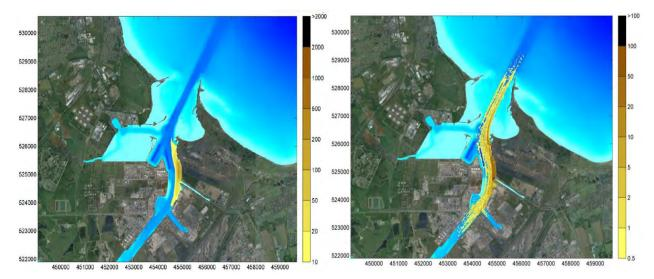
Figure 27.3 Predicted increase in SSC (left) and deposition on the seabed (right) as a result of the Anglo American Harbour Facilities (Royal HaskoningDHV, 2014)
