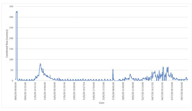
Figure 6.15 Flow measured through the Tees Barrage June – July 2020 (Canal and Rivers Trust, 2020)
