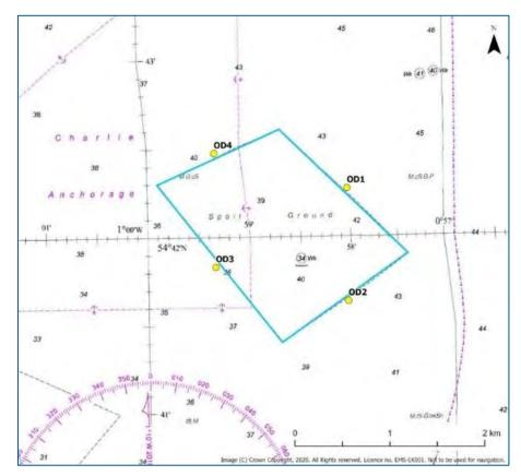
Figure 6.67 Location of points around the offshore disposal site used for of timeseries analysis of changes in SSC and sediment deposition
