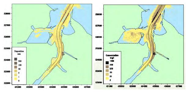
Figure 27.2 Predicted increase in SSC (left) and deposition on the seabed (right) as a result of the NGCT (Royal Haskoning, 2006)
