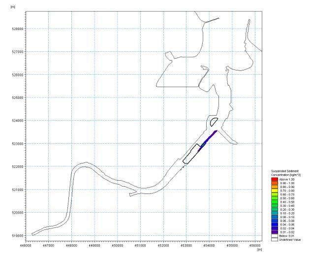
*Figure 6.35* (*Plot D*) – *Plume of enhanced SSCs arising from dredging activities during Stage 1 of the capital dredging programme*
