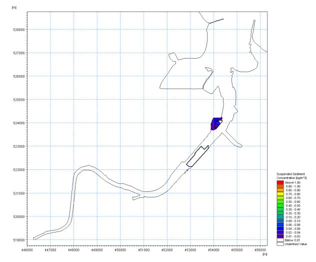
*Figure 6.45* (*Plot A*) – *Plume of enhanced SSCs arising from dredging activities during Stage 4 of the capital dredging programme*
