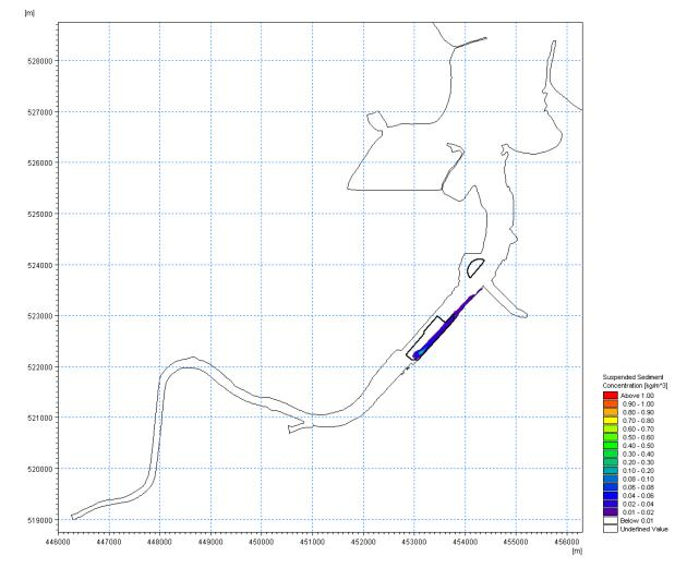
*Figure 6.32* (*Plot A*) – *Plume of enhanced SSCs arising from dredging activities during Stage 1 of the capital dredging programme*
