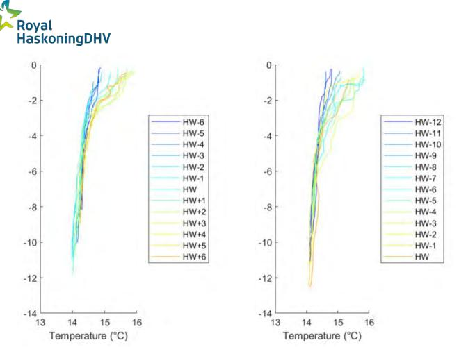
*Figure 6.17 Measured hourly temperature profiles at the centre of transect T8 during neap (left) and spring (right) tides in July 2020*
