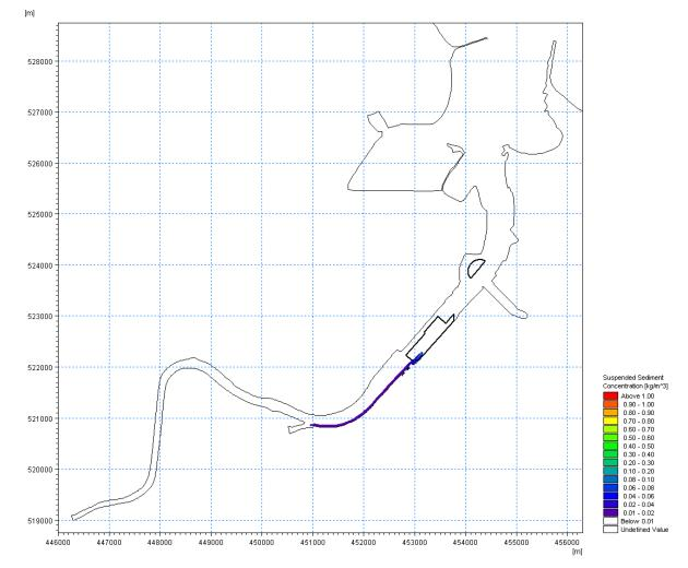
*Figure 6.33* (*Plot B*) – *Plume of enhanced SSCs arising from dredging activities during Stage 1 of the capital dredging programme*
