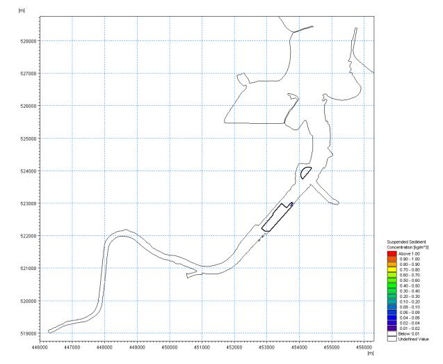
*Figure 6.42* (*Plot C*) – *Plume of enhanced SSCs arising from dredging activities during Stage 3 of the capital dredging programme*
