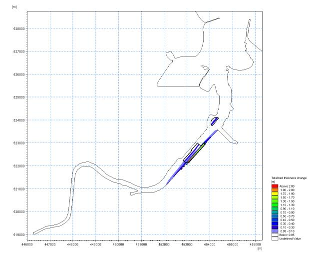
Figure 6.50Maximum riverbed thickness change due to sediment deposition arising from dredging<br/>activities during Stages 1 - 4 inclusive of the capital dredging programme
