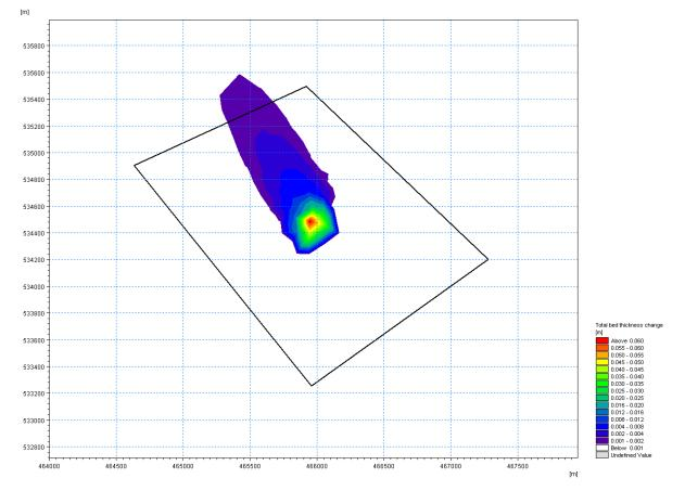
Figure 6.65Maximum sea bed thickness change due to sediment deposition arising from one disposalevent during Stage 1 of the capital dredging programme – local scale
