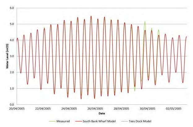
Figure 6.7 Comparison of Measured and Modelled Tidal Elevation at Tees Dock Tide Gauge
