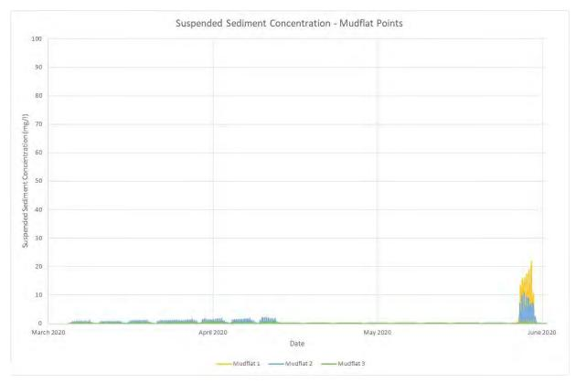
Figure 6.54 Timeseries of changes in SSC at the mudflat monitoring points
