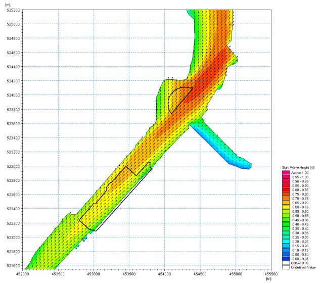
Figure 6.25 Local wind-generated saves for 1 in 100 year return period coming from south-southwest (210 degrees) (proposed scheme)
