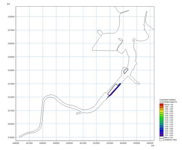
*Figure 6.34* (*Plot C*) – *Plume of enhanced SSCs arising from dredging activities during Stage 1 of the capital dredging programme*
