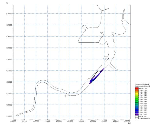
*Figure 6.37* (*Plot A*) – *Plume of enhanced SSCs arising from dredging activities during Stage 2 of the capital dredging programme*
