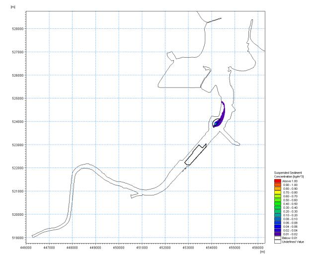
*Figure 6.46* (*Plot B*) – *Plume of enhanced SSCs arising from dredging activities during Stage 4 of the capital dredging programme*
