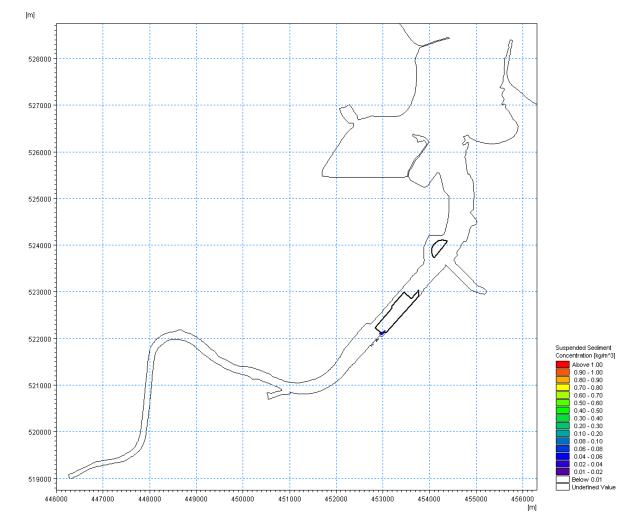
*Figure 6.40* (*Plot A*) – *Plume of enhanced SSCs arising from dredging activities during Stage 3 of the capital dredging programme*
