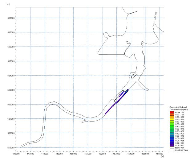
*Figure 6.38* (*Plot B*) – *Plume of enhanced SSCs arising from dredging activities during Stage 2 of the capital dredging programme*
