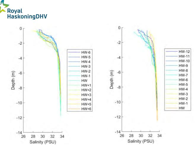
Figure 6.16Measured hourly salinity profiles at the centre of transect T8 during neap (left) and spring<br/>(right) tides in July 2020
