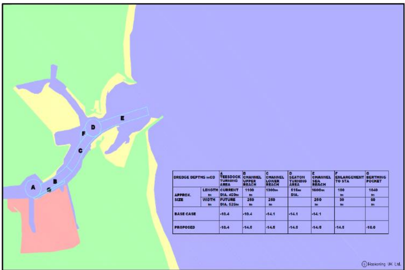
Figure 1 Dredge areas for the NGCT (the small scale and localised dredging at QEII Berth required for relocation of the Riverside Ro-Ro is not shown on this figure)
