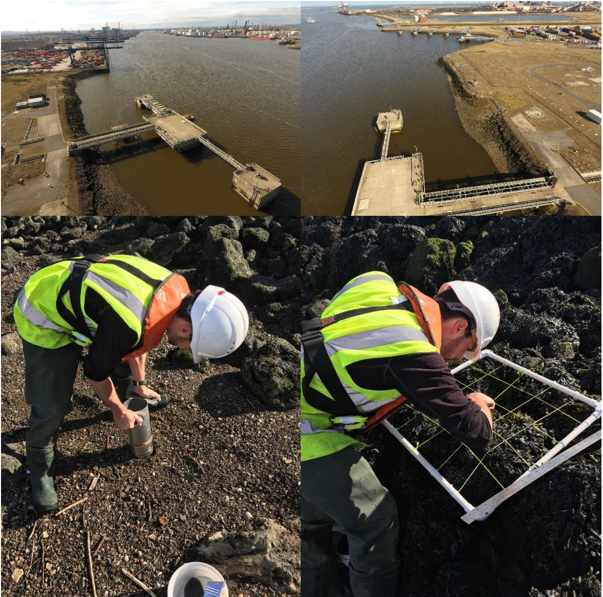
Plate 3. Top left: Aerial image of intertidal survey area and Teesport Container Terminal. Top right: Aerial image of intertidal survey area and the Riverside Ro-Ro ferry terminal. Bottom left: Soft sediment 0.01 m 2 core sampling. Bottom right: Hard substratum 0.25 m 2 quadrat sampling.
