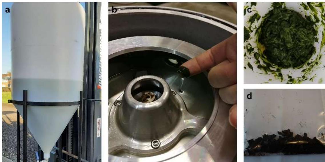
Figure 9 - End of second experiment including: a) collection of the microalgal biomass in a vessel before centrifugation; b) centrifuge with microalgal biomass being collected; c) wet microalgal biomass; d) dried microalgal biomass.
