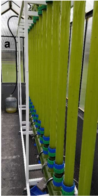
Figure 8 - MISTY system: a) Varicon Aqua Phyco-Lift photobioreactor standing inside of a greenhouse; b) The greenhouse in wintertime with an outside temperature of 0.94 °C and an inside temperature of 9.31 °C.
