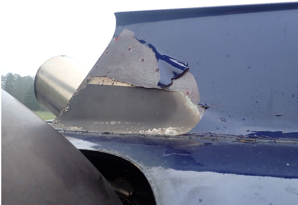
Figure 2 Paint blistering on engine cowling adjacent to right engine inboard exhaust tube
