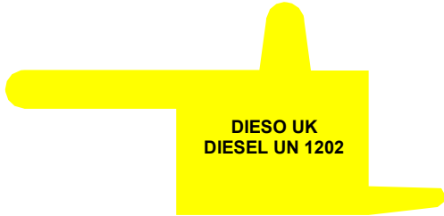
Figure 2.1.2.6 – DIESO UK, Depot Filled. NSN: 40R 9905-99-767-3032 ( note 1 ) Pantone colour 1235C ( note 3a ) BS 381C colour 356 Golden Yellow ( note 3b )
