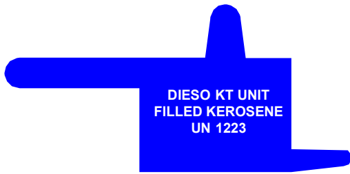
Figure 2.1.2.12 – DIESO KT, Unit Filled. (note 2) NSN: 40R 9905-99-474-5691 (note 1) Pantone colour 302C (note 3a) BS 381C colour 109 Middle Blue (note 3b)
