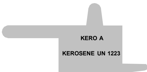
Figure 2.1.2.10 – KERO A, Depot Filled. NSN: 40R 9905-99-297-6209 ( note 1 ) Pantone colour 444C ( note 3a ) BS 381C colour 637 Medium Sea Grey ( note 3b )
