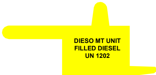
Figure 2.1.2.9 - DIESO MT, Unit Filled. NSN: 40R 9905-99-270-7856 ( note 1 ) Pantone colour 1235C ( note 3a ) BS 381C colour 356 Golden Yellow ( note 3b )
