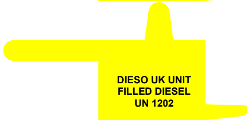
Figure 2.1.2.7 – DIESO UK, Unit Filled. NSN: 40R 9905-99-433-3092 Pantone colour 1235C ( note 3a ) BS 381C colour 356 Golden Yellow ( note 3b )
