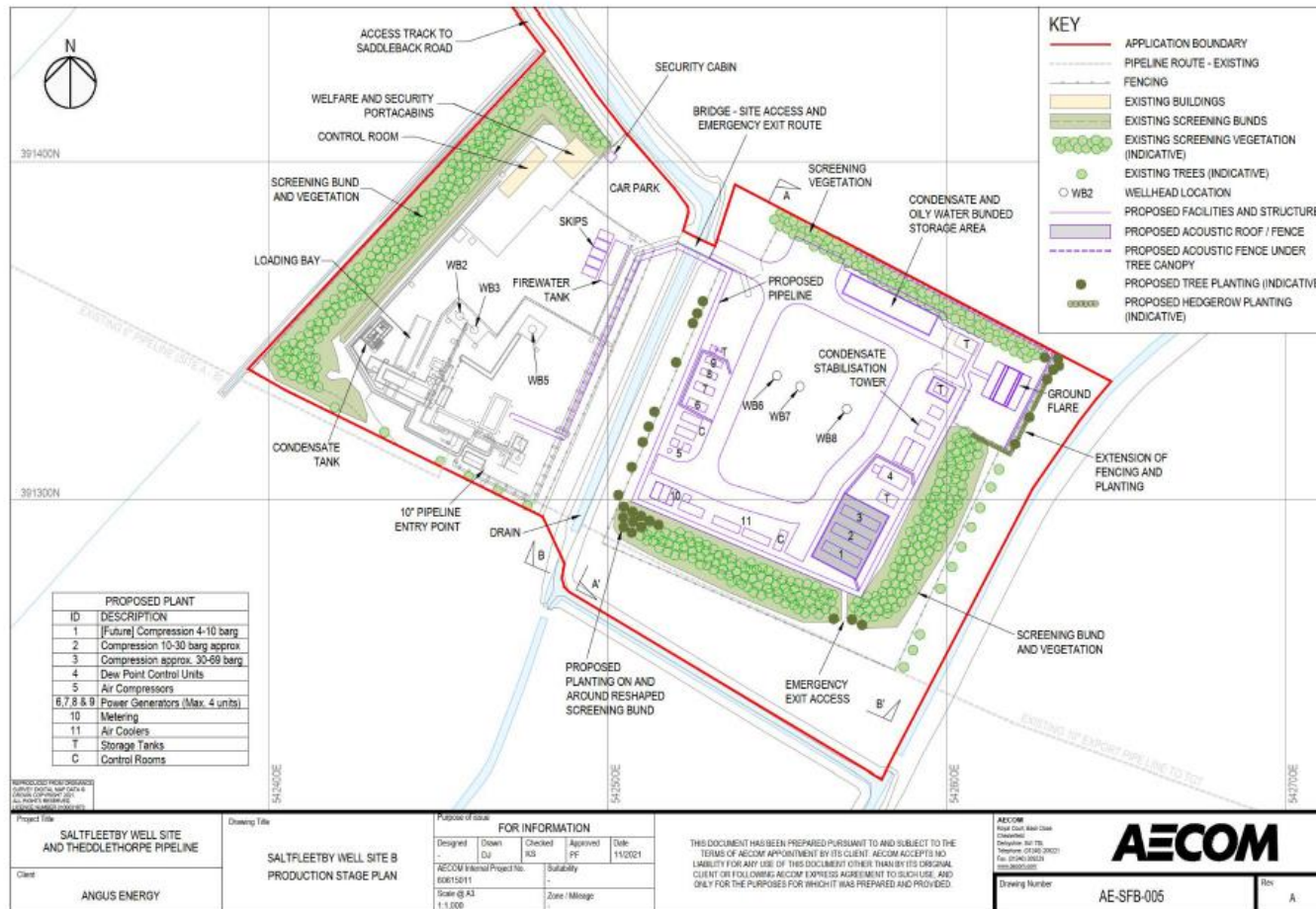
Angus En Figure 2: Proposed Site Layout (Production Phase) of the Saltfleetby B Well site Issued 22/03/2022 Page 8 of 81
