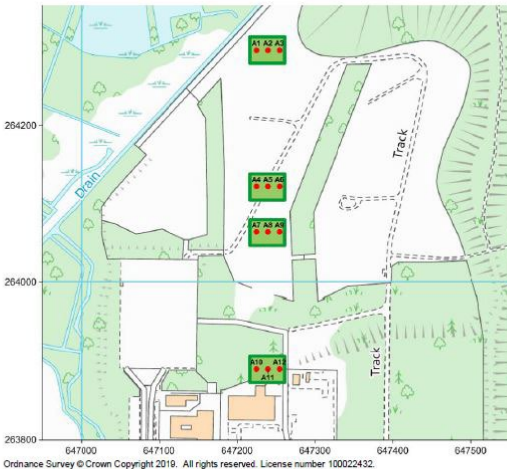
Figure 1 Proposed location of the purpose-built concrete buildings, each containing 2 EDGs and one UDG. Units A1, A2 and A3 are closest to the adjacent Minsmere to Walberswick Heaths and Marshes SAC, Minsmere-Walberswick SPA and Minsmere-Walberswick Ramsar. Taken from Fig. 12C.1, NNB GenCo, 2020a
