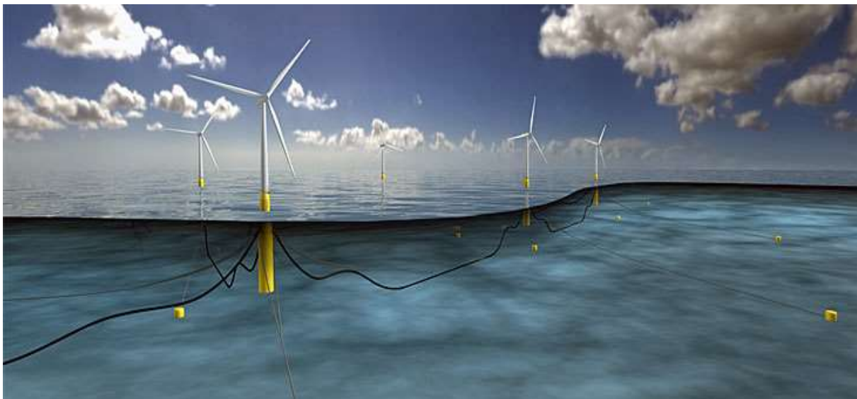
Figure 5: Schematic of completed Hywind pilot project
