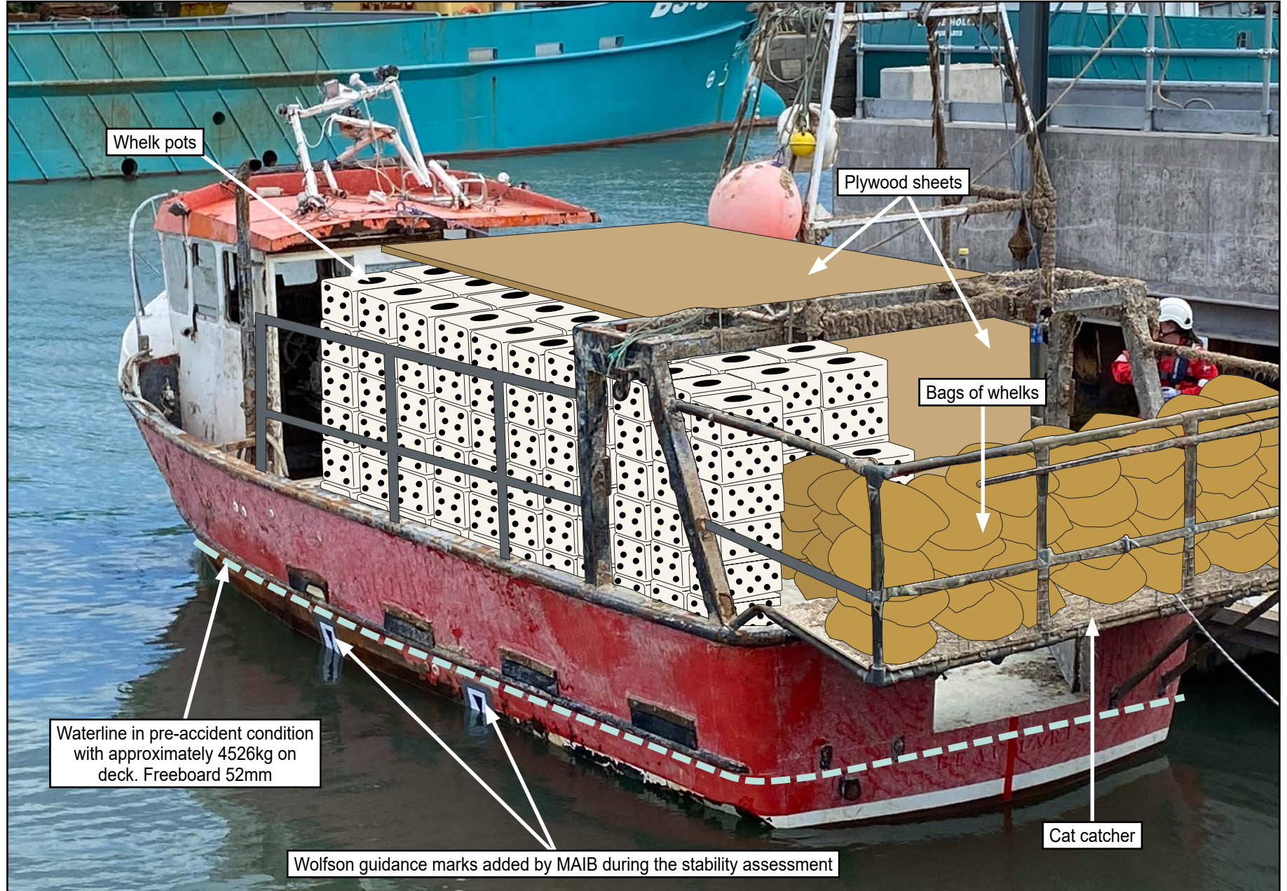
Figure 20: Possible loading condition of Nicola Faith before the accident
