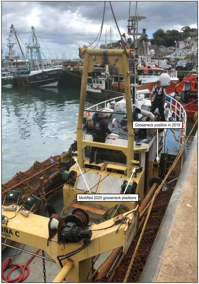
Figure 11: Derrick gooseneck position after the 2020 move
