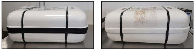
Figure 15: New liferaft, showing addition of manufacturer's black tape (left) and *Joanna C*'s repacked liferaft (right)
