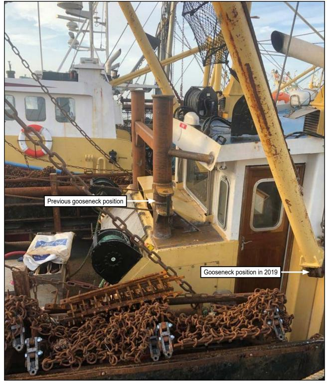
Figure 10: Derrick gooseneck position after the 2019 modifications
