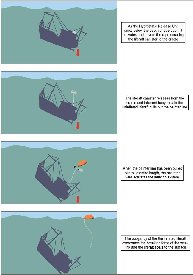
Figure 12: Operational sequence of a Hydrostatic Release Unit
