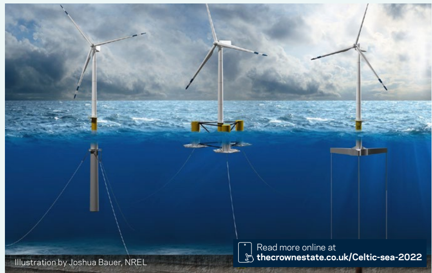
Illustration by Joshua Bauer, NREL Floating wind foundation types (l to r): Spar, Semisubmersible, Tension leg platform.
