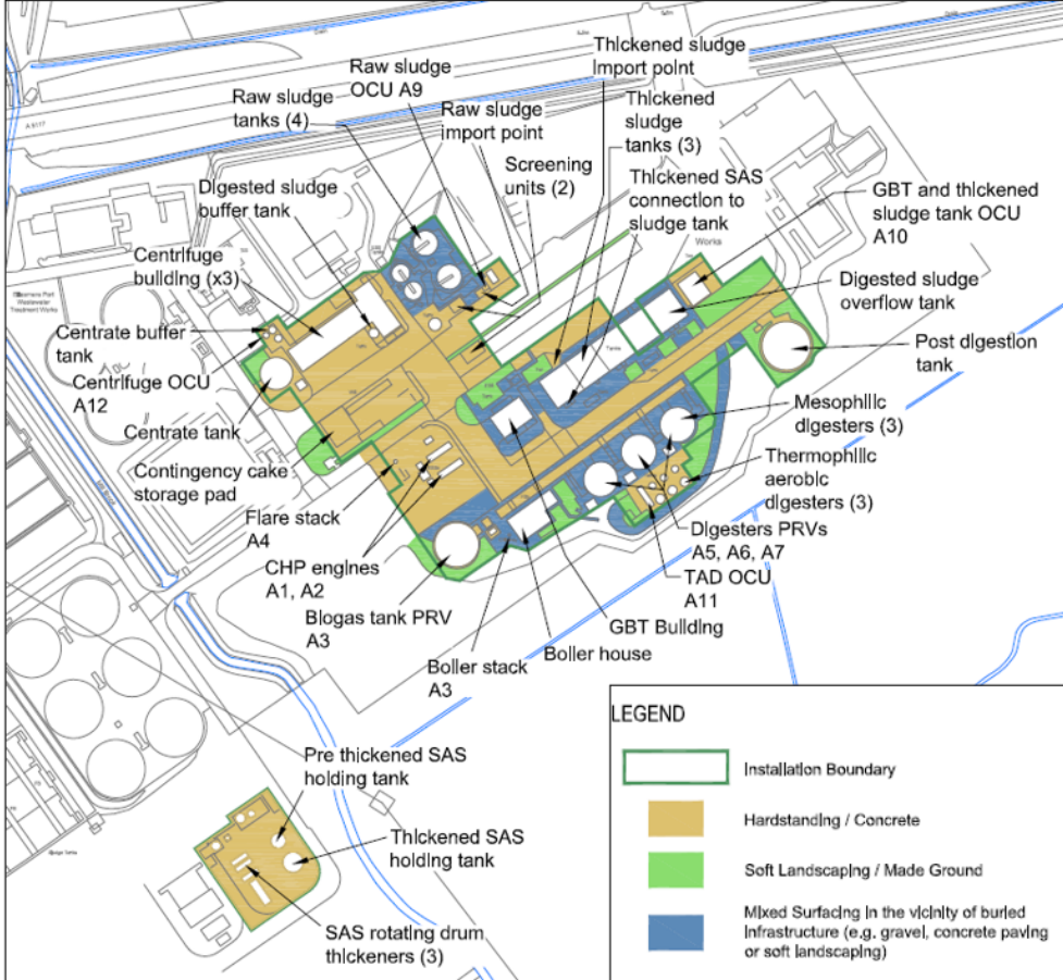
Figure 2 – Site surfacing plan
