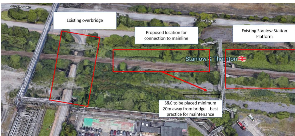
Figure 3-3 – Proposed location for Switches & Crossings (S&C) for connection to mainline at Stanlow
