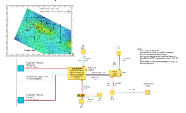
Figure 13: Endurance Phase 1 subsea development
