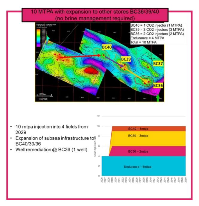
Figure 11: Path to 10 MTPA (Phase 2) from Phase 1 (4 MTPA at Endurance) with the expansion into additional stores (BC36/39/40) to add 6 MTPA capacity (no brine would be expected).
