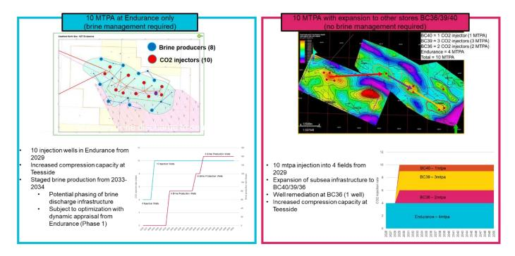
Figure 10: Path to 10 MTPAa (Phase 2) from Phase 1 (4 MTPAa at Endurance). Option 1 would involve expanding Endurance to 10 MTPAa with brine production facility while option 2 would require expansion into additional stores (BC36/39/40) to add 6 MTPAa capacity (no brine production would be expected).
