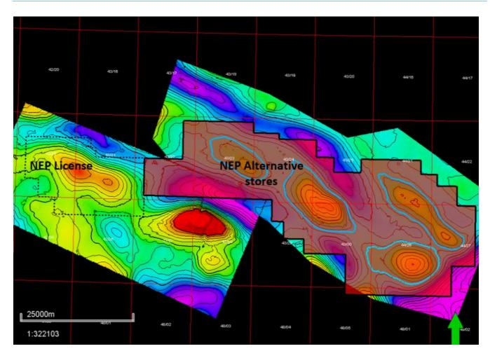
Figure 4: Potential store license boundaries covering the additional Bunter structures identified as suitable for CO2 storage near Endurance (BC40, BC39, BC36, and BC37).
