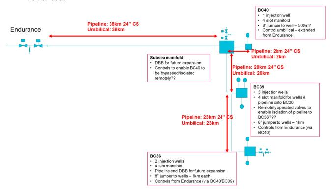
Figure 12: Notional subsea expansion from Endurance to BC40, BC39, and BC36 (subsea system will have the ability to be connected to BC37 as well to support future phases).
