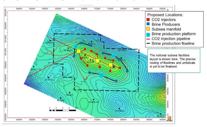
Figure 8: Notional 10 MTPA development with 10 CO2 injectors and 8 brine producers (surface discharge)
