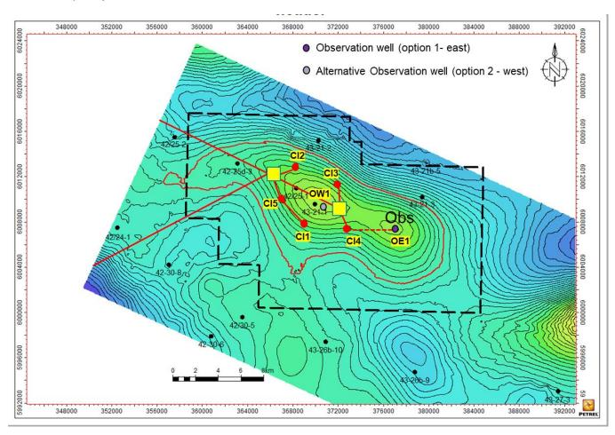
Figure 5: Phase 1 subsea development with 5 CO2 injectors and 1 observation well.
