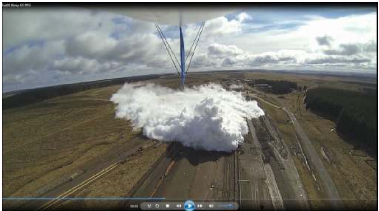
Figure 31(j): Aerial View at Time 210 s from Rupture
