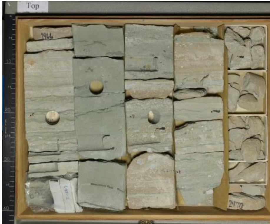
Figure 3-3: Well 48/29-A1, core 1, depth 2964 – 2970 ft (Upper Bunter interval).
