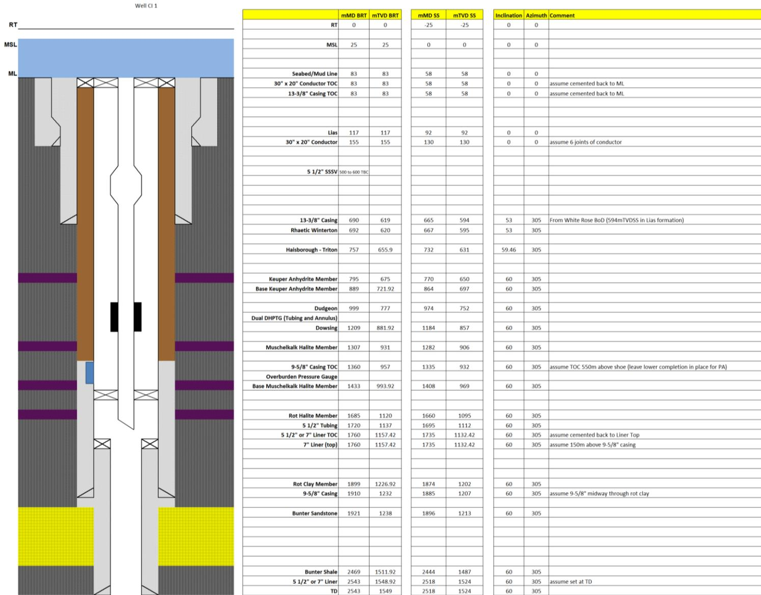
Figure 10 Wellbore Schematic (Well CI4 drilled from drill centre DC1 – clustered subsea layout)
