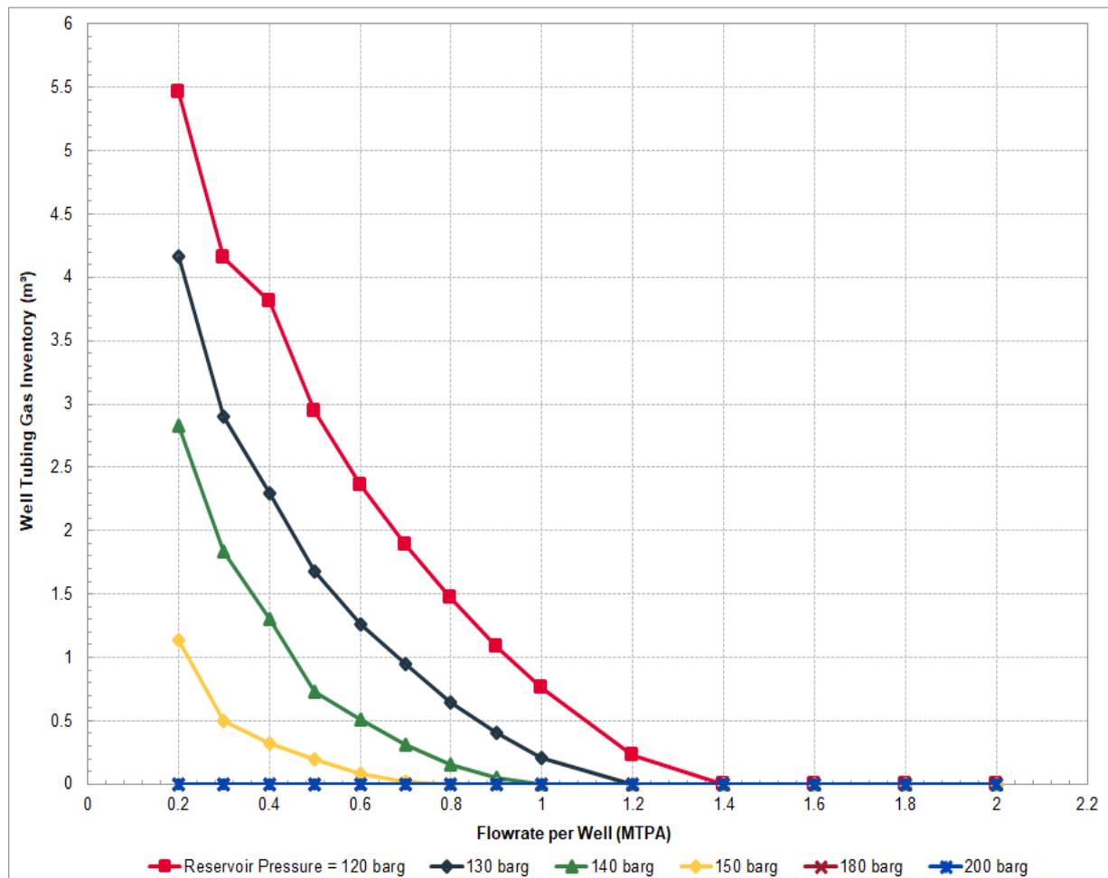
**Figure 55 Gas Pocket Volume vs. Injection Rate and Reservoir Pressure**
