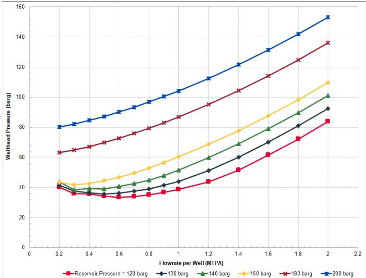
**Figure 51 Steady State Flowing Wellhead Pressures vs. Flowrate and Reservoir Pressure**
