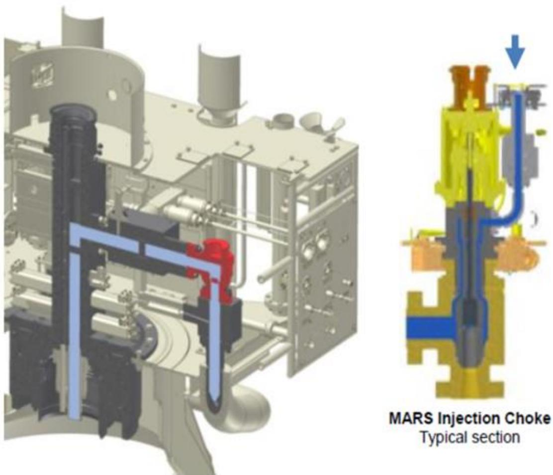
**Figure 74 MARS Choke Insert for Water Wash Access**
