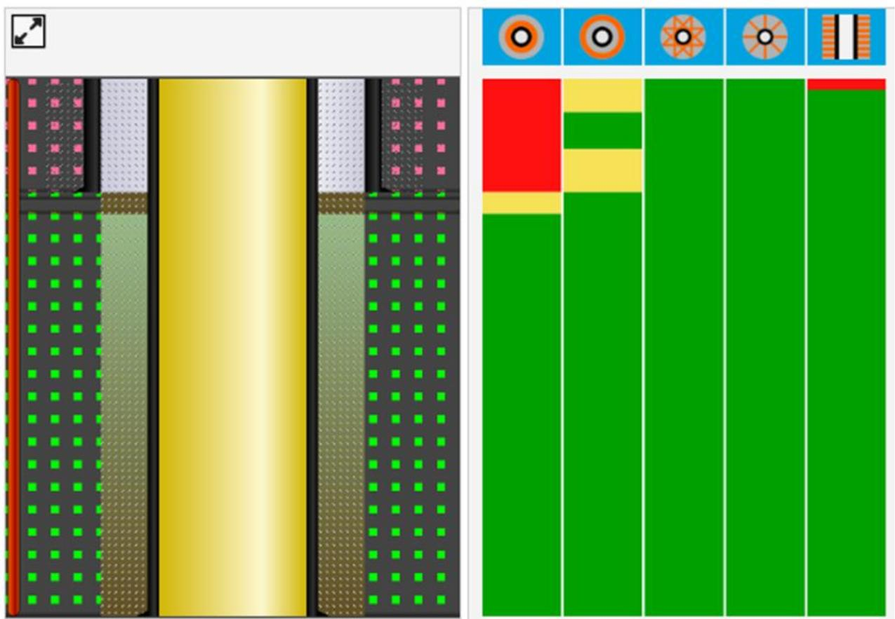
Figure 39 Case B: 5 1/2" Liner in 8 1/2" Open Hole with 15.3 ppg Cement
