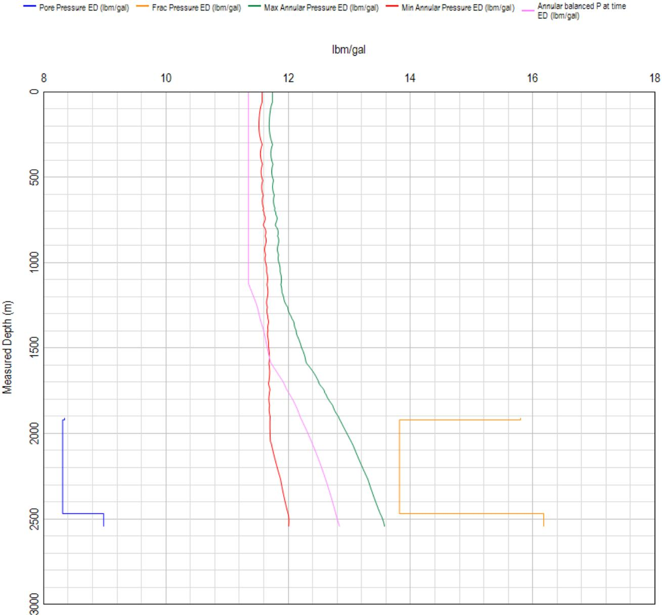
Figure 35 Liner Cement Job ECD
