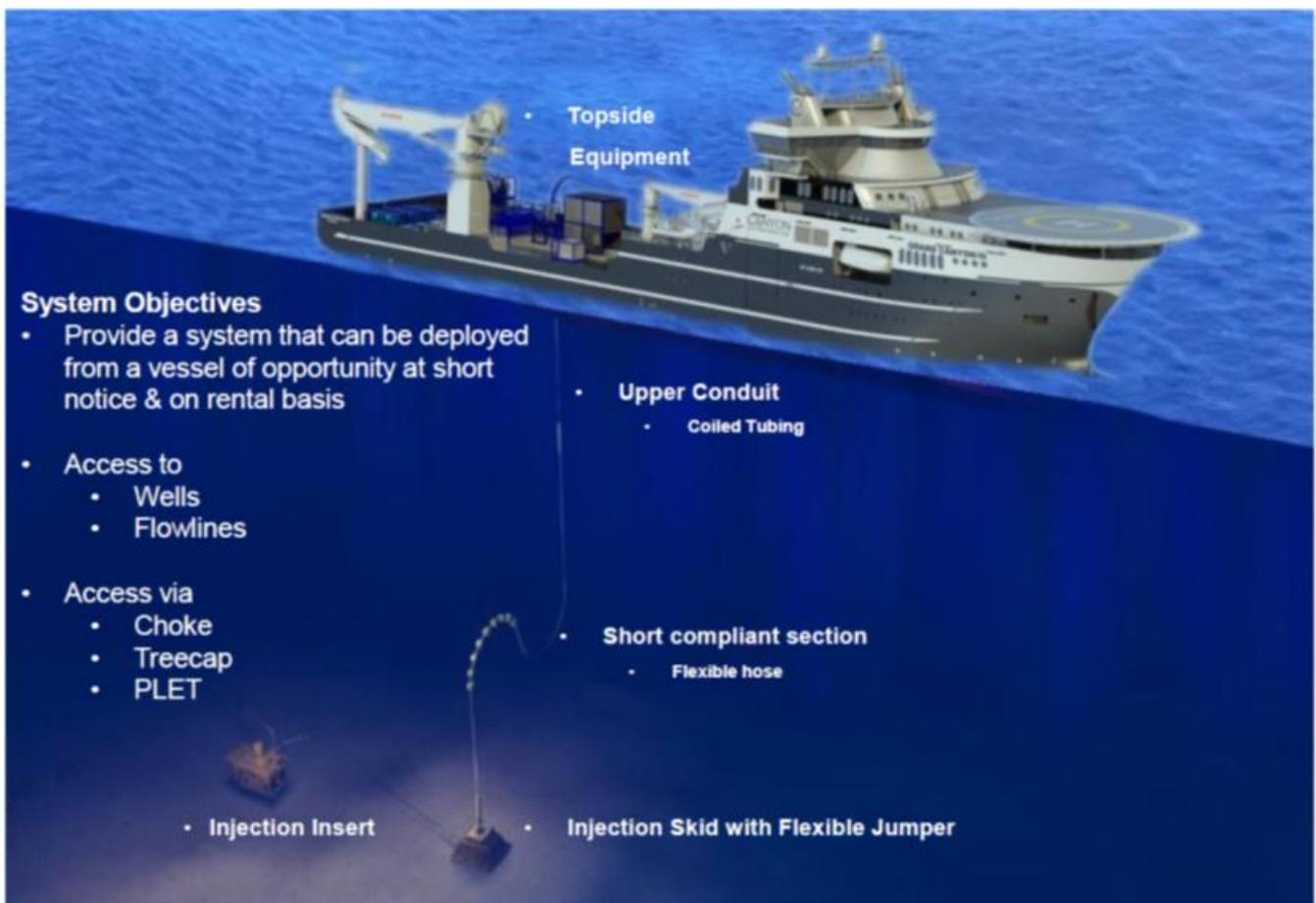
Figure 75 MARS System Operation from Vessel
