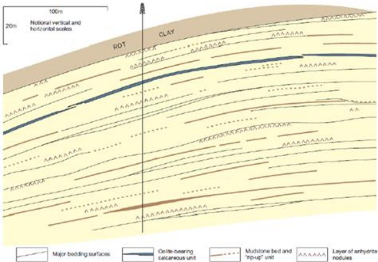
Figure 60 Cross Section at 42/25d-3 Potential Geometry of Permeability Baffles and Barriers<sup>10</sup>
