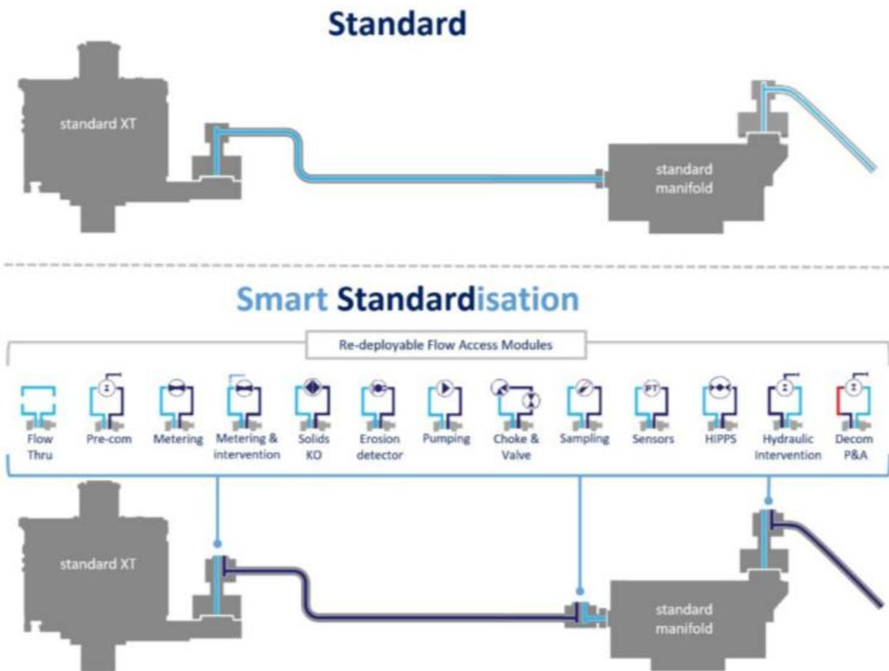
Figure 77 ENPRO External Fluid Access System (manifold or tree)
