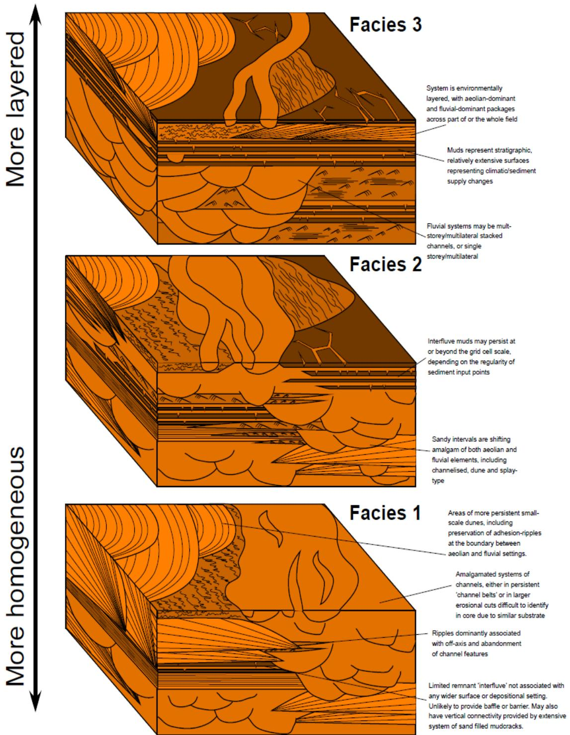
Figure 57 Representation of the Bunter Sandstone Depositional Environment around 42/25d-3
