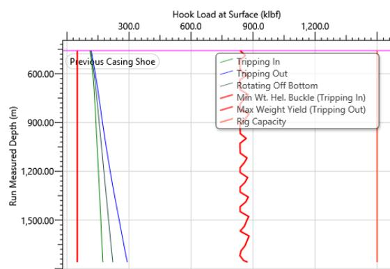
Figure 24 Well CI4 - 9-5/8" Casing Drag Plot
