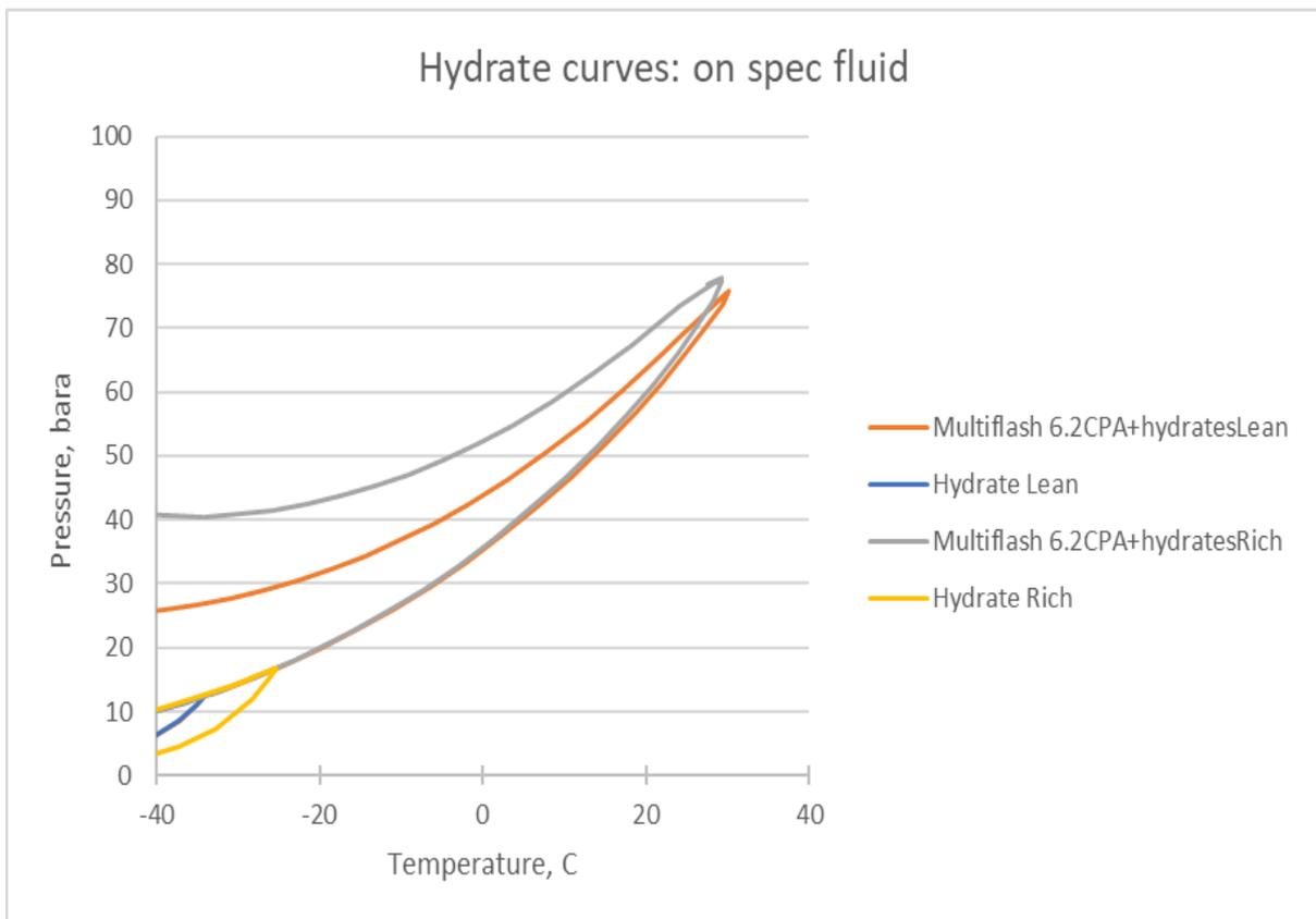
**Figure 48 Phase Envelopes and Hydrate Curves in Contact with Pure Water**
