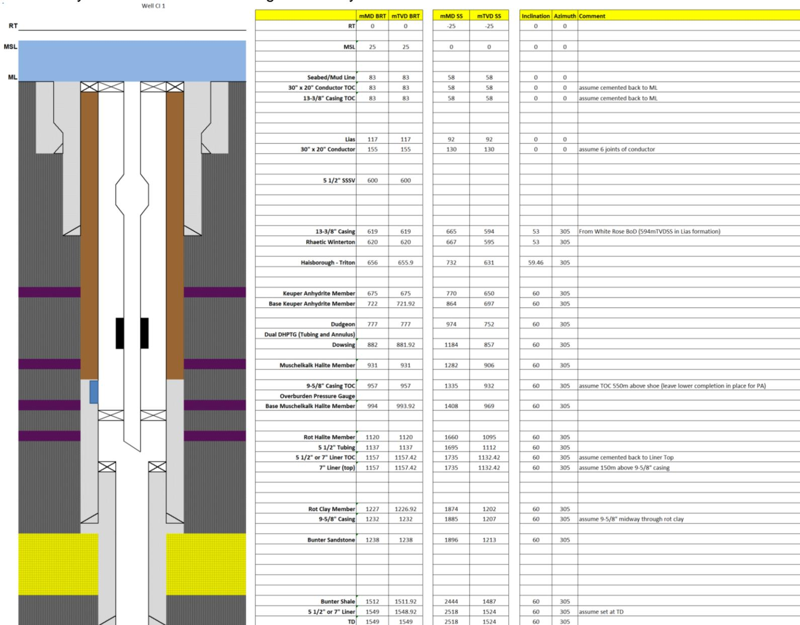
Figure 11 Wellbore Schematic (Well C1 drilled vertically – Distributed subsea layout)
