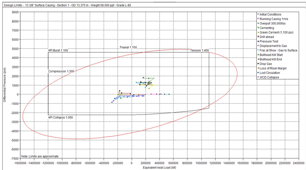
**Figure 31 13-3/8" Surface Casing Design Limits Plot**
