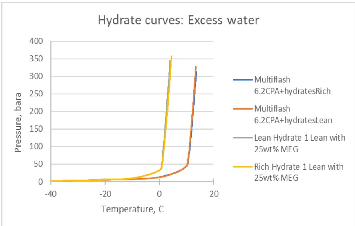
Figure 50 Hydrate Curves for Rich and Lean CO2 with Excess Water, with and without MEG
