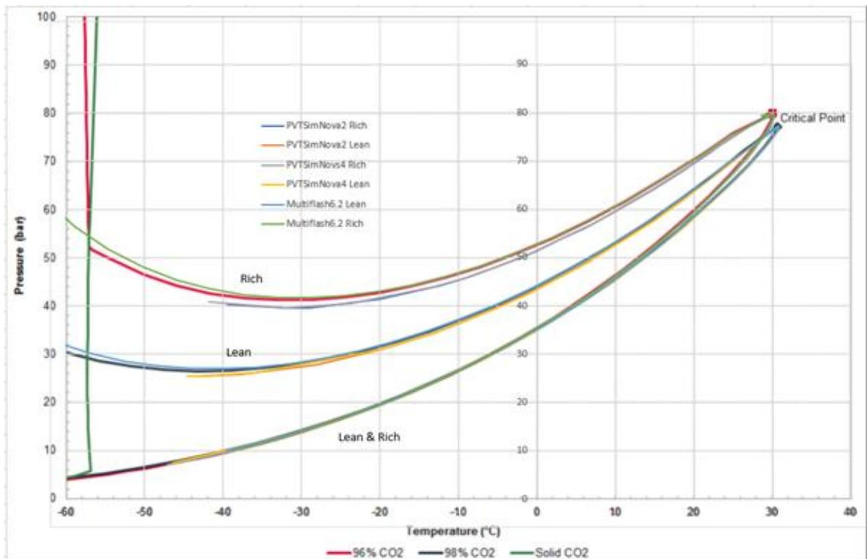
Figure 46 NZT/NEP Specification Phase Envelope for CO<sub>2</sub> Containing Impurities
