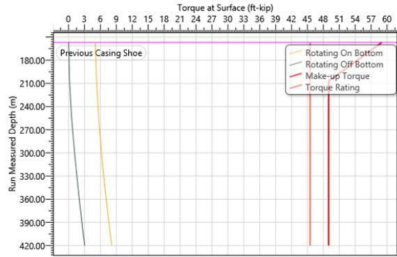
Figure 14 Well CI4 - 17-1/2" Torque Plot
