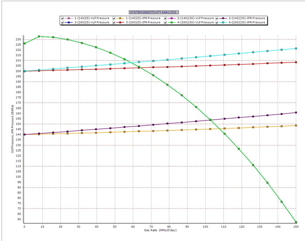
Figure 63 Tubing Performance with 3 1/2" Tailpipe to TD Injecting Mid-Perf at 1950 m MD
