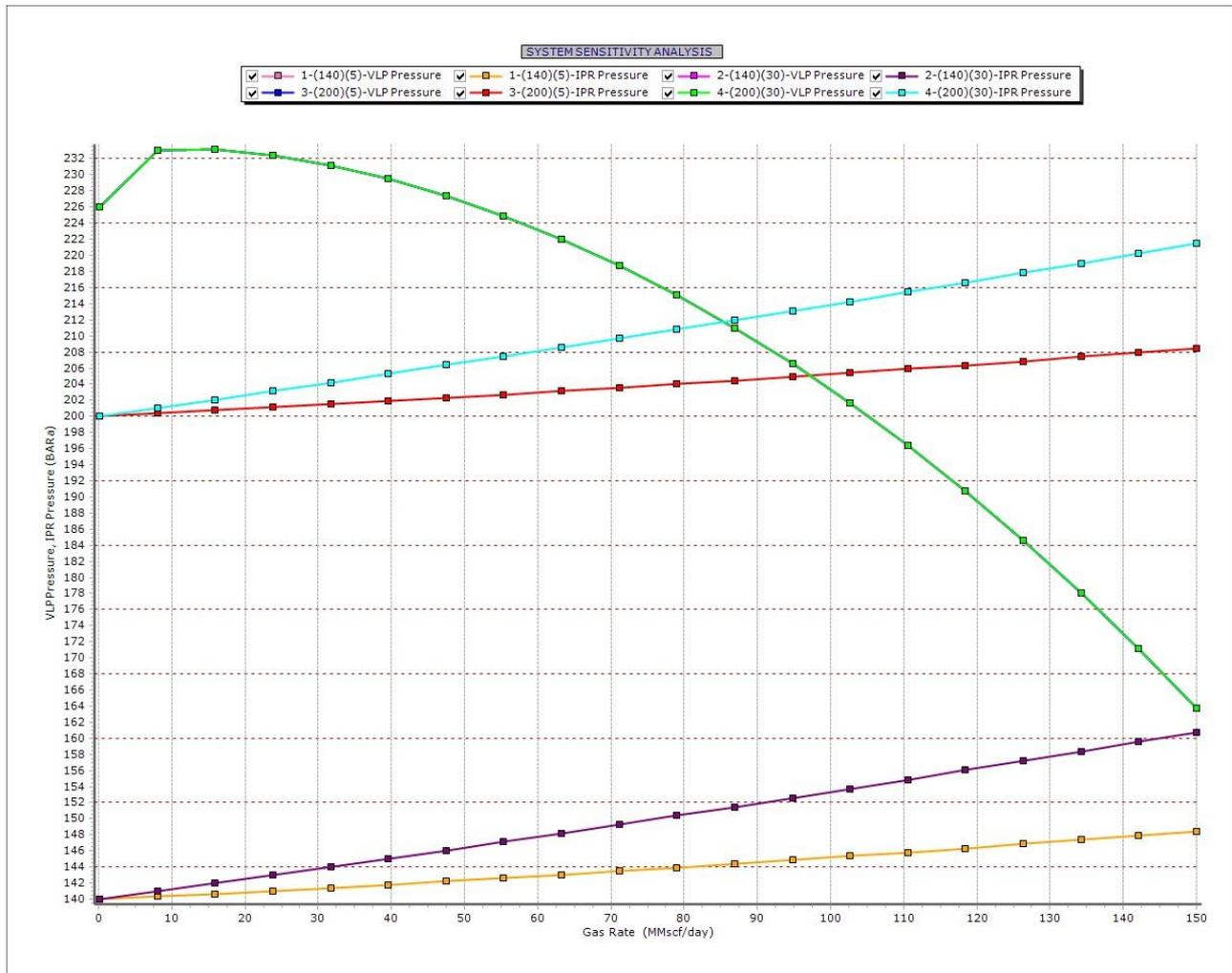
**Figure 62 Tubing Injection Performance (5 1/2” Tubing, WHIP 110 bar, Skin 5-30, Pr 140-200 bar)**
