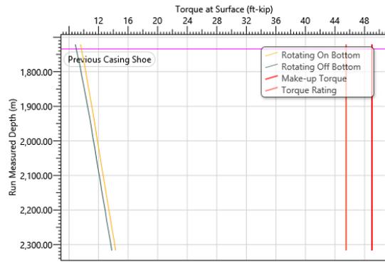
Figure 26 Well CI4 - 8-1/2" Torque Plot
