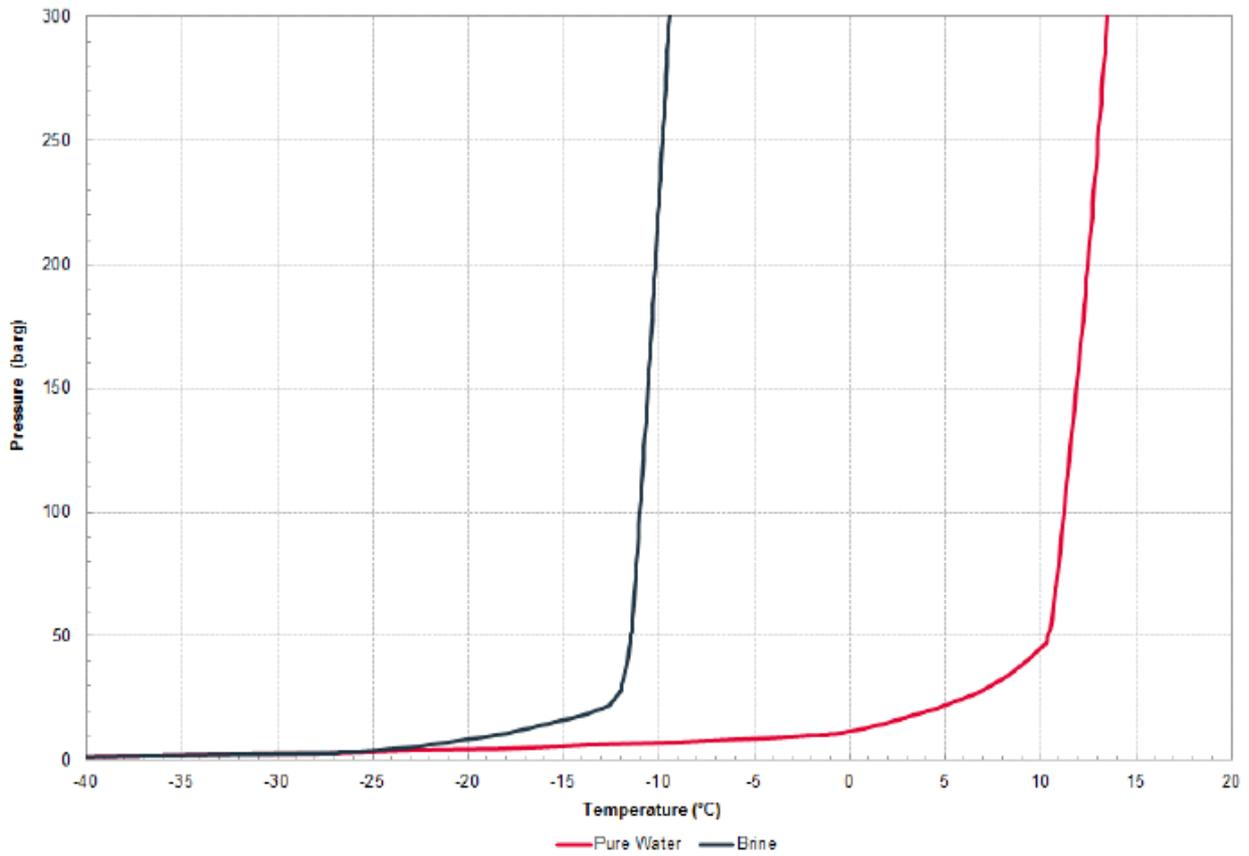
Figure 49 Hydrate Curve for CO2 in Contact with Water or Formation Brine
