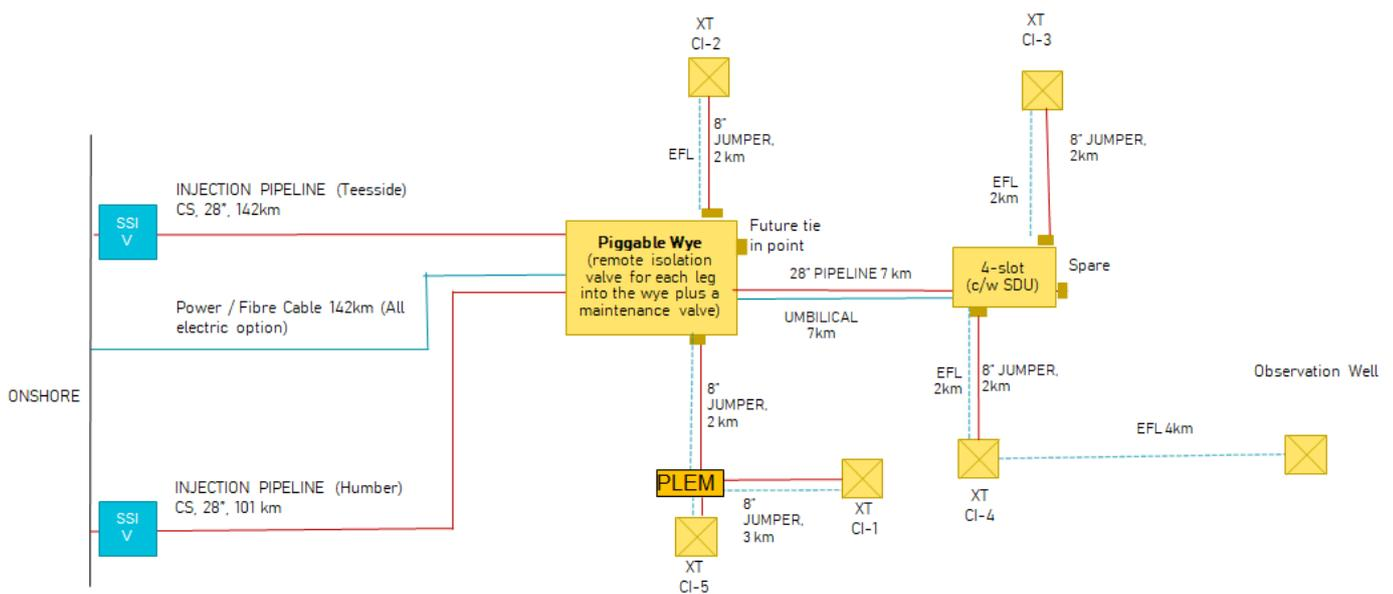
**Figure 73 Distributed Subsea Equipment**
