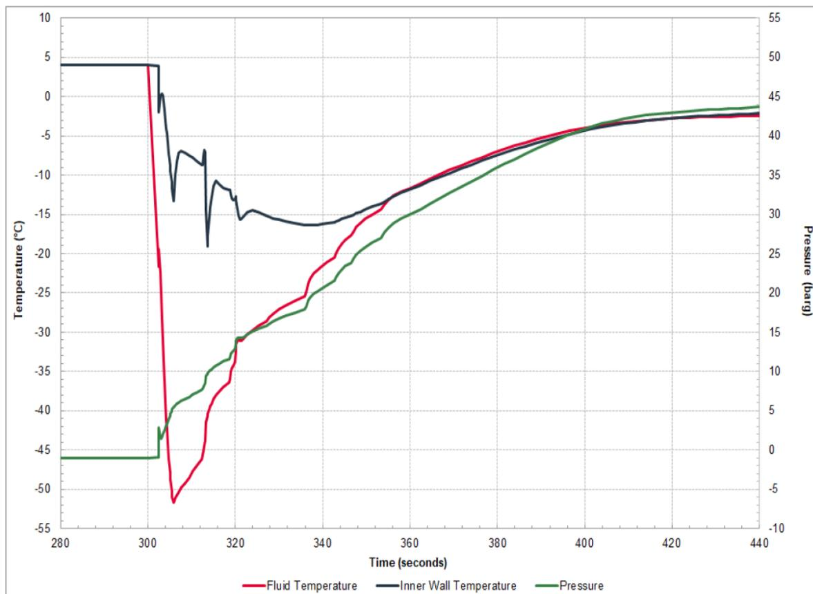
**Figure 54 Wellhead Pressure and Temperature during Restart after Wash-Water Treatment**
