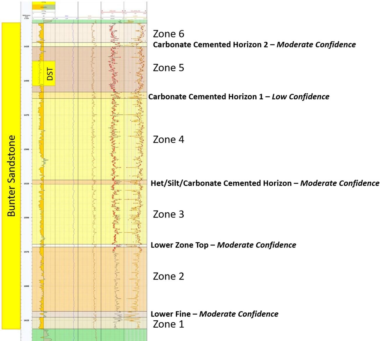
Figure 59 42/25d-3 Log Showing Baffles and Barriers
