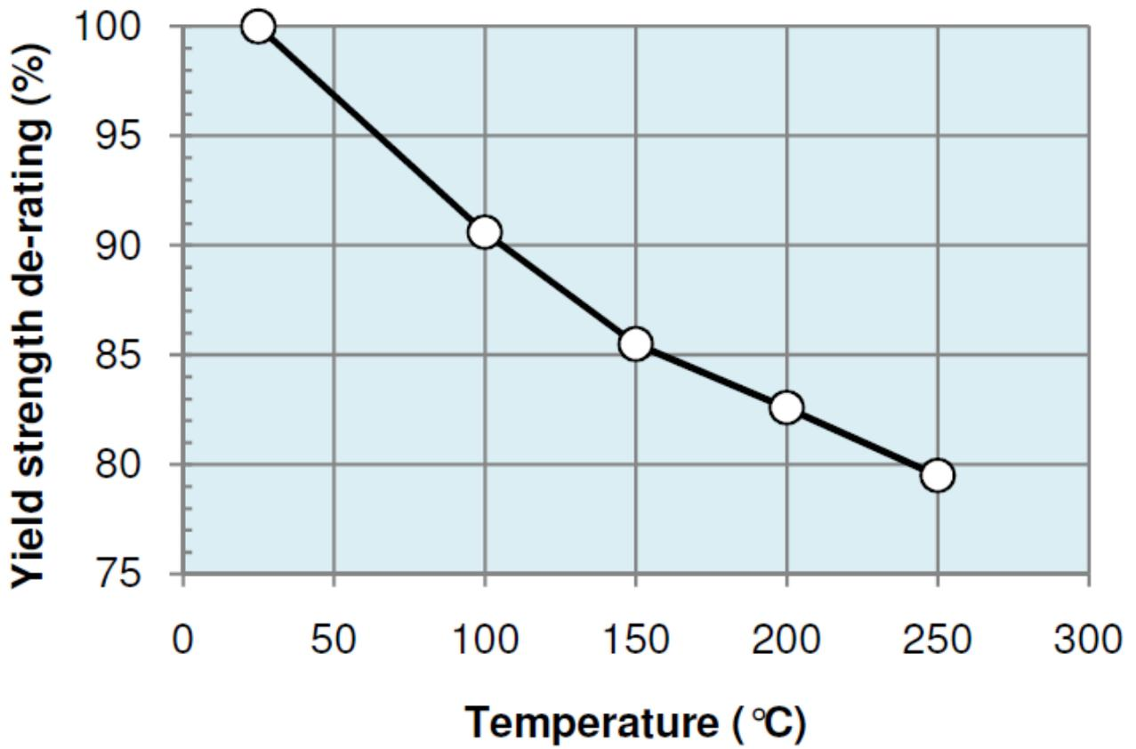
Figure 79 Sumitomo SM25CR-125 Yield Strength Deration with Temperature
