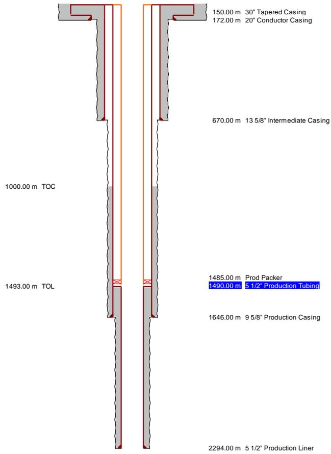
**Figure 78 Well Schematic (RKB 35m)**
