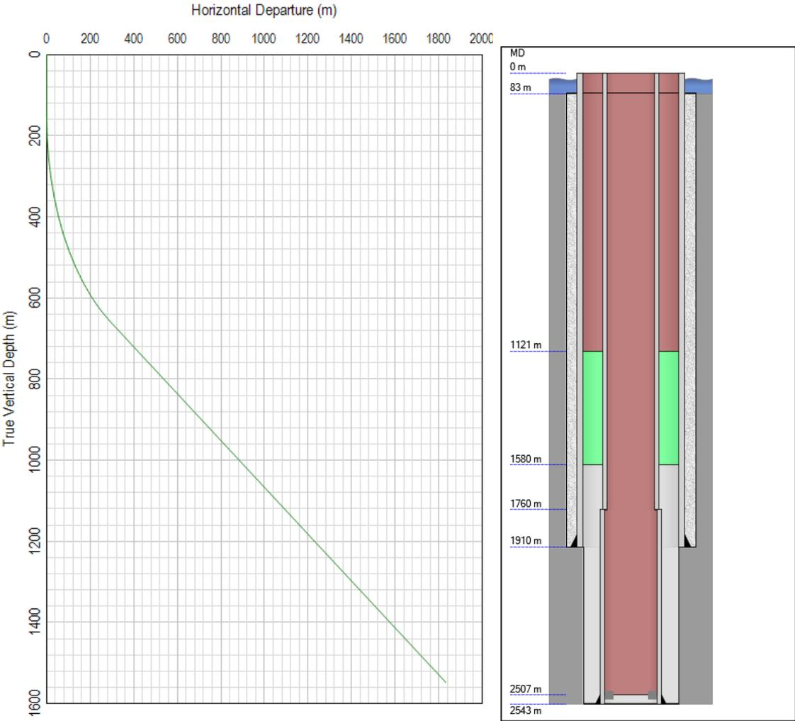
Figure 34 Liner Cement Simulation – Fluid Map
