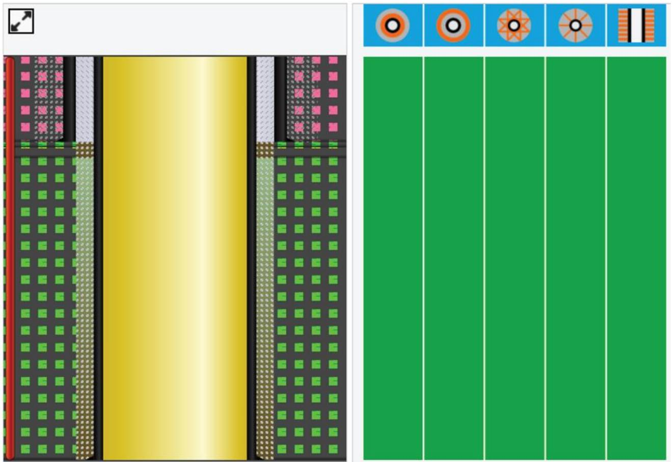
**Figure 40 Case E: 5 1/2" Liner in 8 1/2" Open Hole with 15.3 ppg Cement with Expanding Agent**
