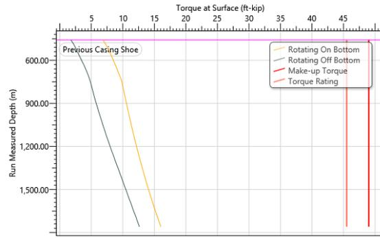
Figure 20 Well CI4 - 12-1/4" Torque Plot
