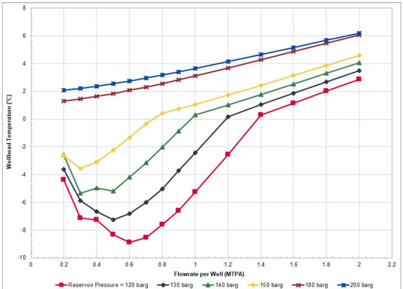
**Figure 52 Steady State Flowing Wellhead Temperature vs. Flowrate and Reservoir Pressure**
