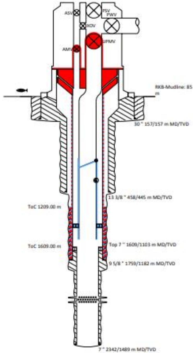
Figure 84 Well Barrier Schematic at Handover
