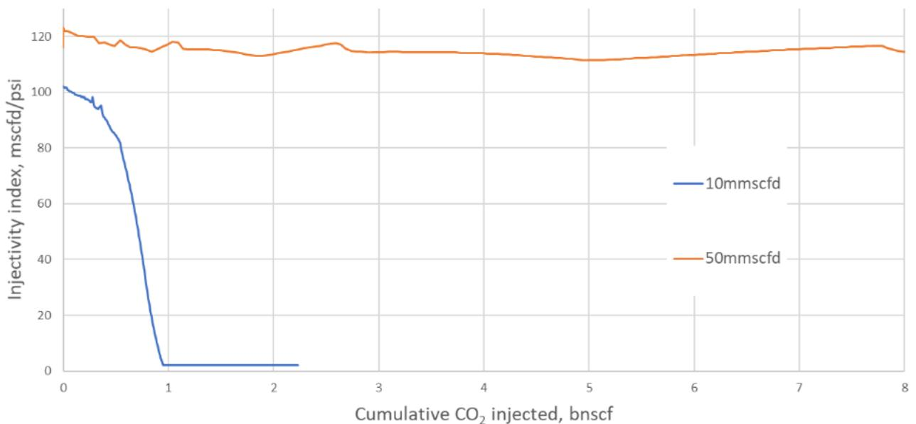
**Figure 47 Injectivity Index for Low and High Injection Rates**
