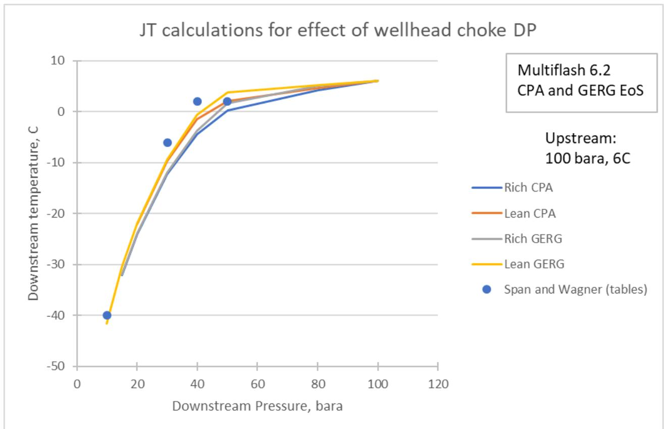
**Figure 53 Flowing Wellhead Temperature vs. Pressure (100 bara and 6 deg C Arrival)**
