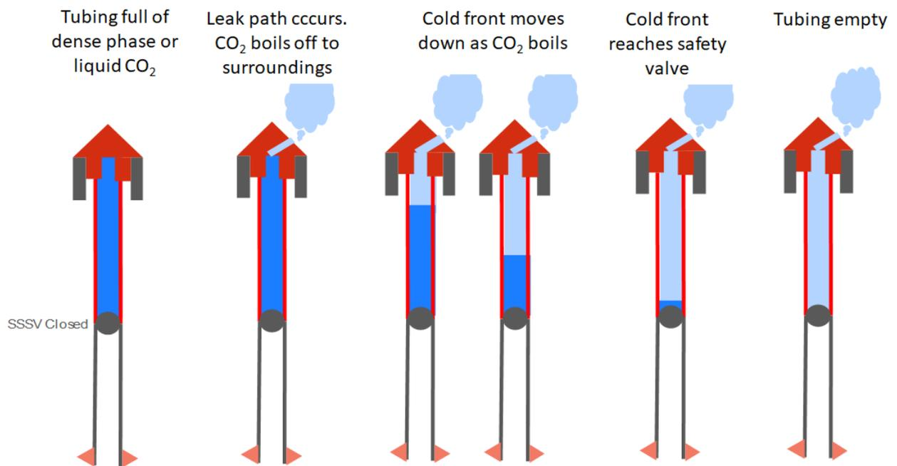
Figure 56 CO<sub>2</sub> Depressurisation with Loss of Primary Containment<sup>8</sup>
