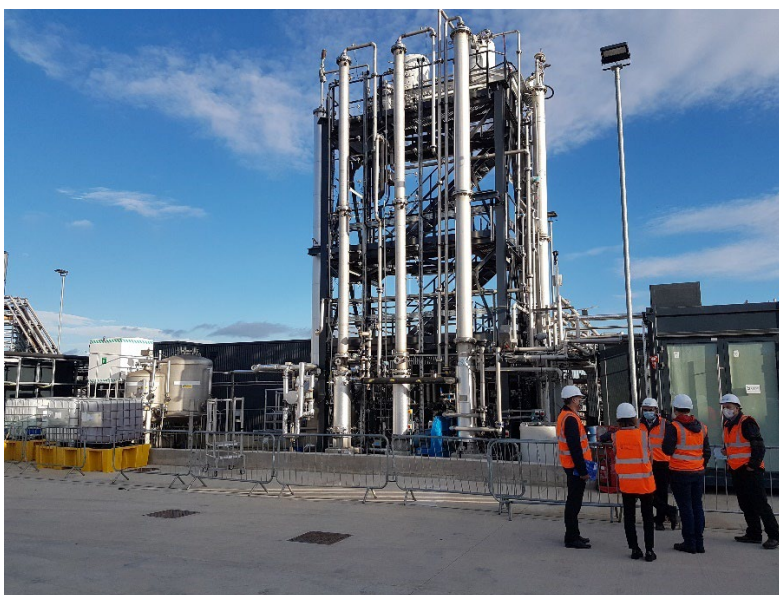
Figure 6. Pilot scale amine capture plant, Translational Energy Research Centre (TERC), University of Sheffield ( www.terc.ac.uk )
