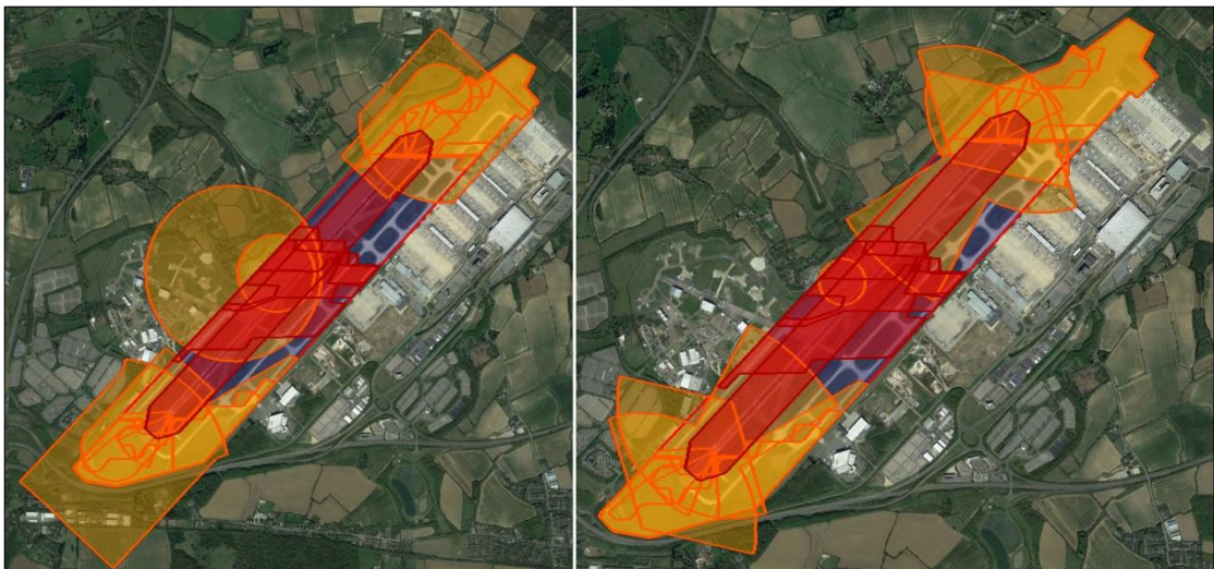
Figure 3 - Area available (blue) when moderate and hard constraints are considered (left - ICAO, right - CAP)
