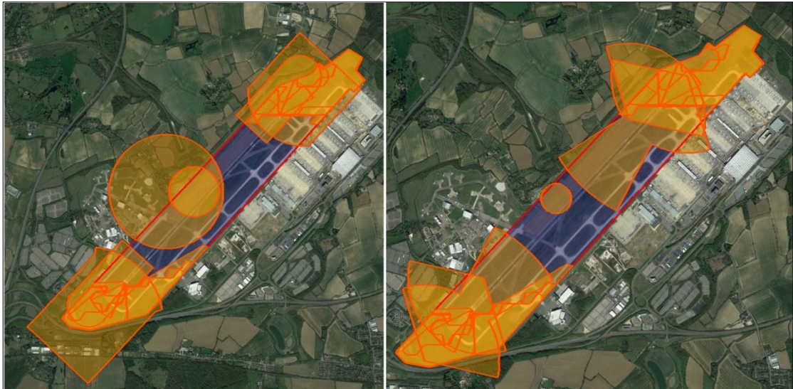
Figure 2 - Area available (blue) when moderate constraints are considered (left - ICAO, right - CAP)
