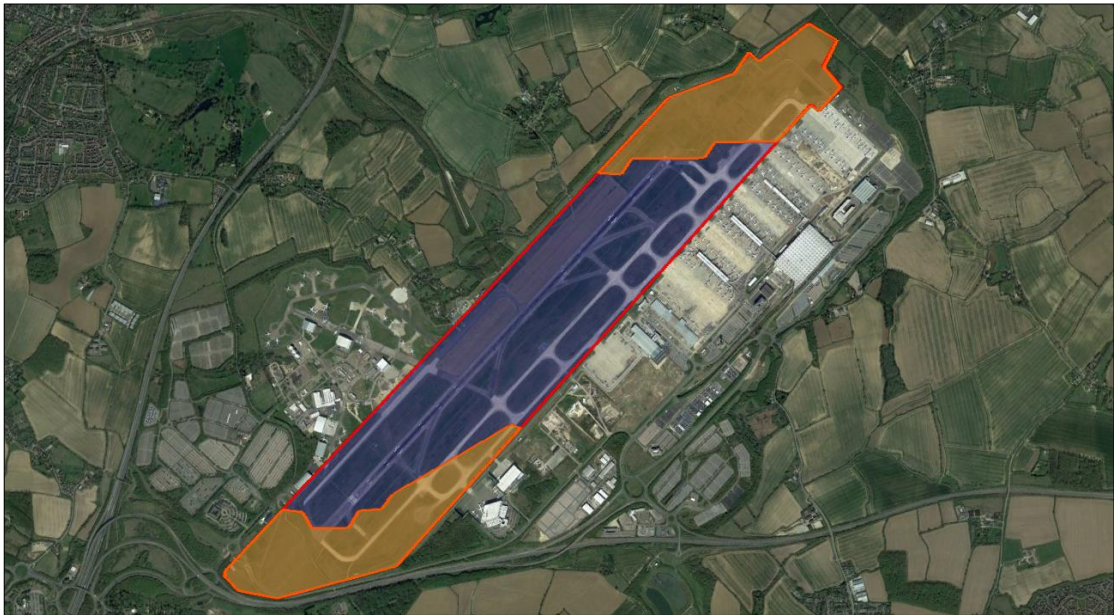
Figure 28 - Solar reflections towards aircrafts approaching at London Stansted Airport for panels oriented 170deg
