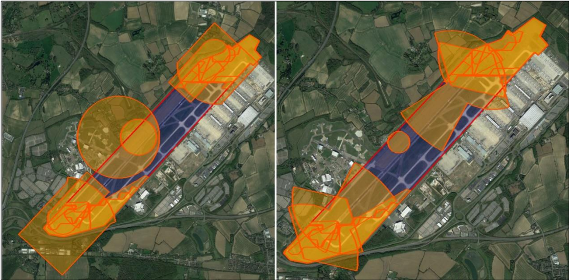
Figure 33 – Area available (blue) when moderate constraints are considered (left – ICAO, right – CAP)
