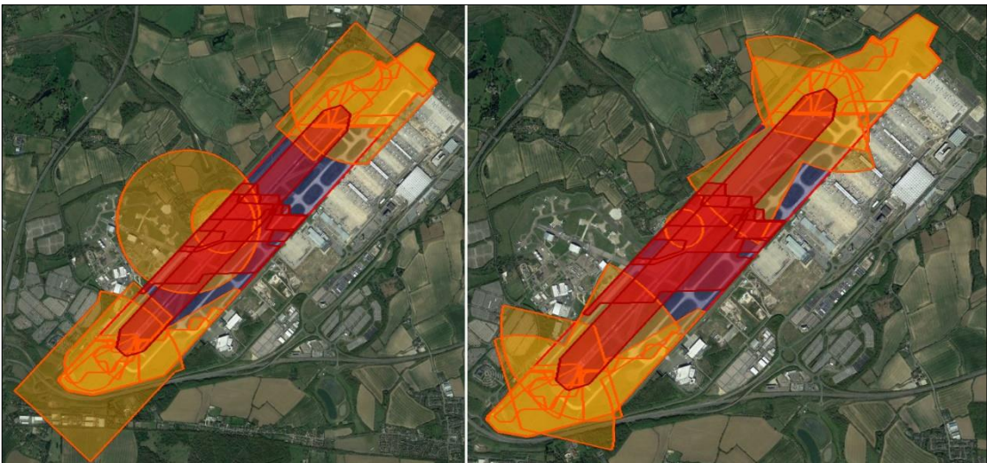
Figure 34 – Area available (blue) when moderate and hard constraints are considered (left – ICAO, right – CAP)
