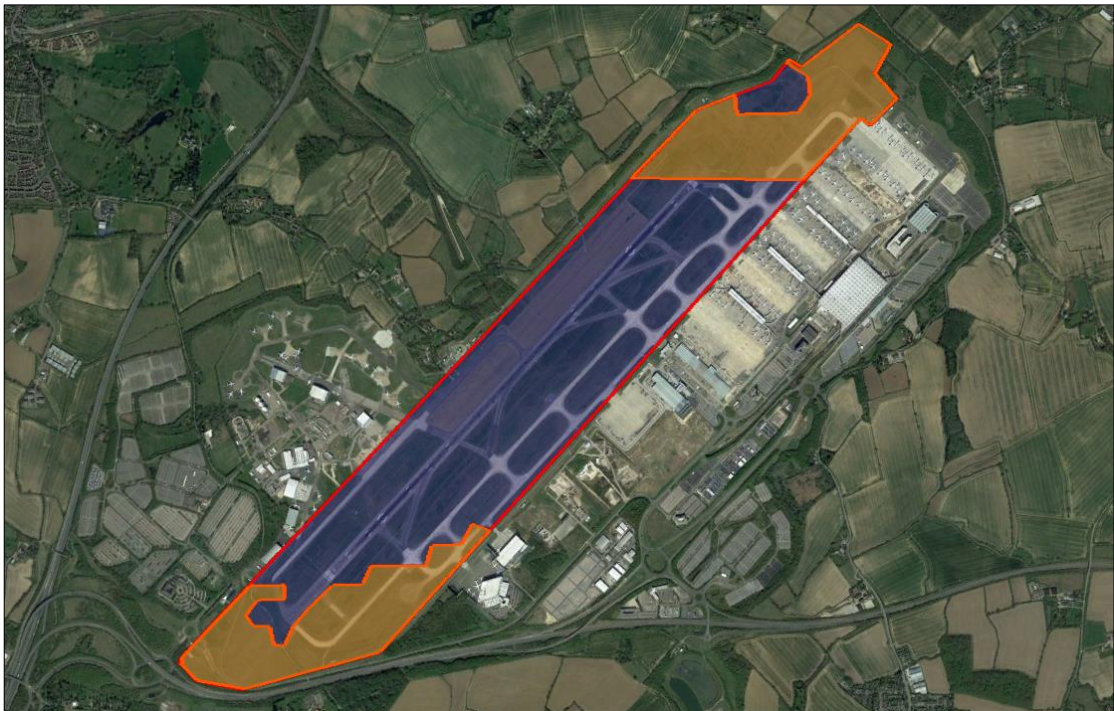
Figure 29 - Solar reflections towards aircrafts approaching at London Stansted Airport for panels oriented 180deg
