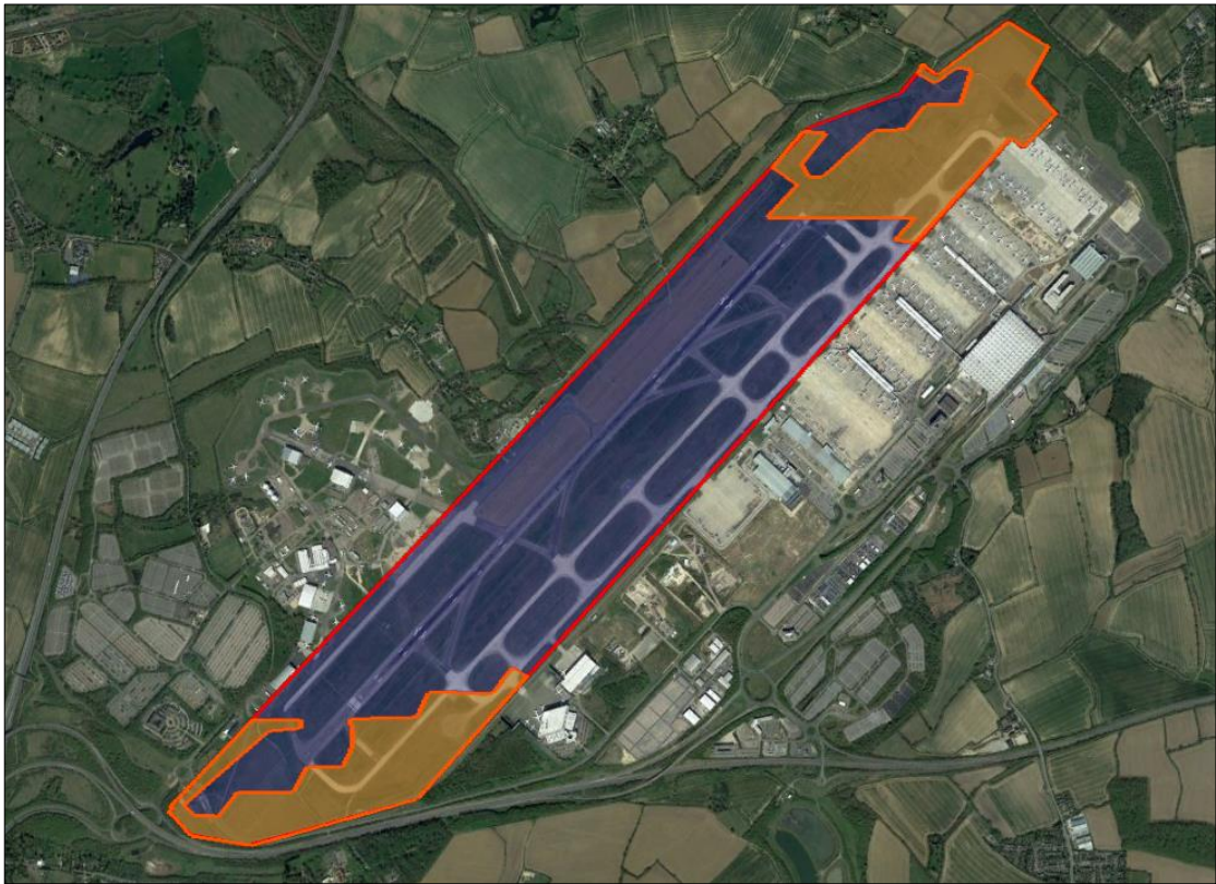
Figure 30 – Solar reflections towards aircraft approaching at London Stansted Airport for panels oriented 190deg
