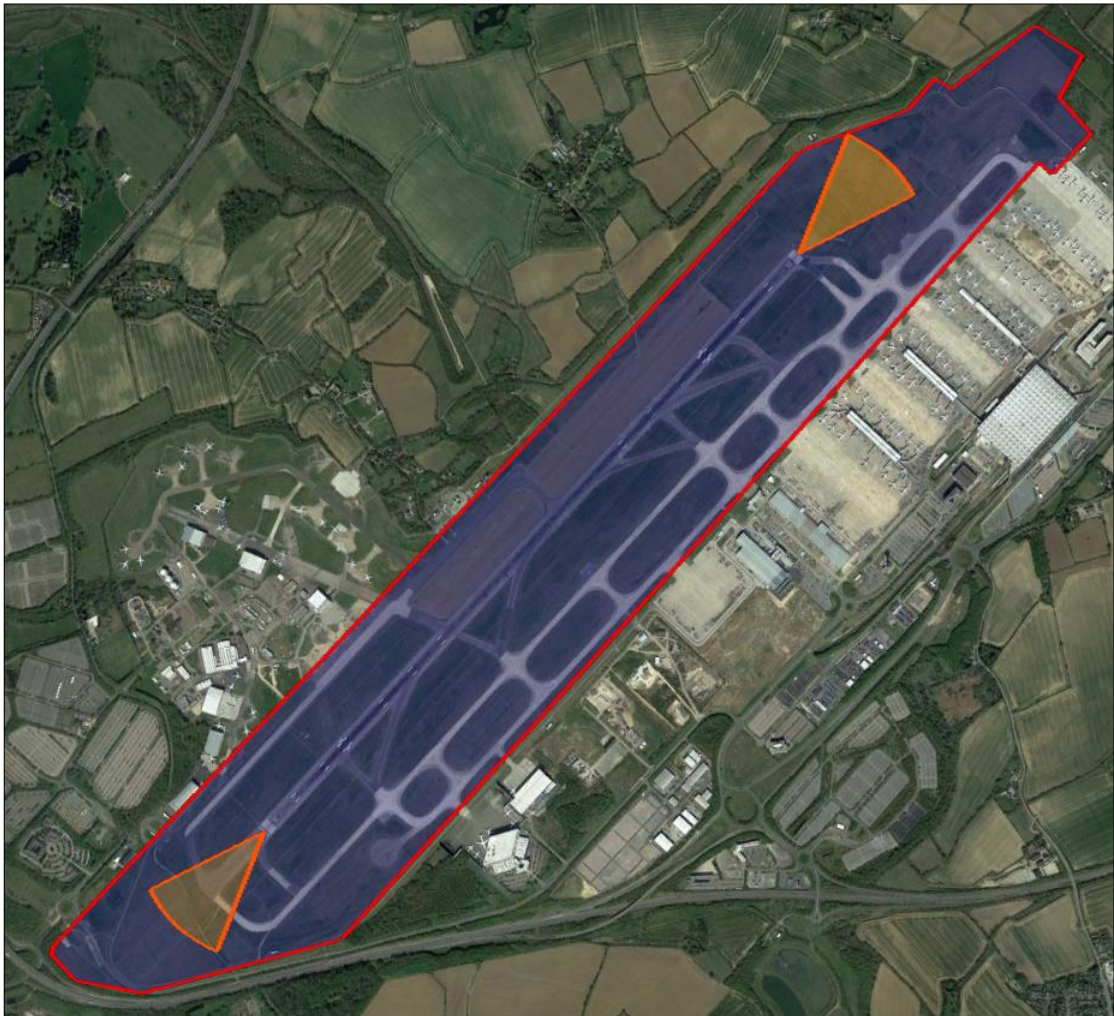
Figure 11 - Jet blast buffer areas where panels should not be installed (orange areas)
