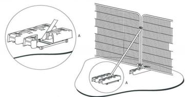
b) Stabilizer strut mounted on block tray
