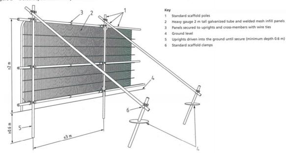
Figure 3 Examples of above-ground stabilizing systems
