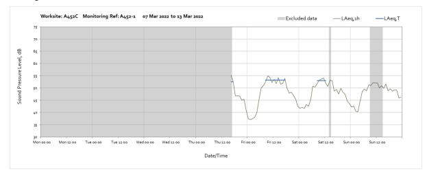
Note: Missing data between 00:00 on 7<sup>th</sup> March and 16:00 on 10<sup>th</sup> March was due to system error which required the meter to be reset. This was identified during maintenance visit and is currently under investigation.
