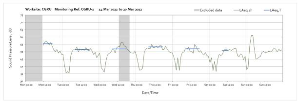
Note: Missing data between 00:00 and 10:00 on 14<sup>th</sup> March was due to a system glitch that required the monitor to be reset.
