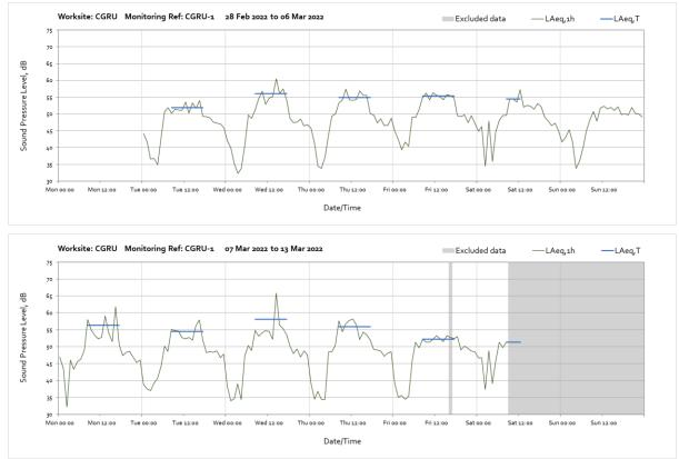
Note: Missing data between 09:00 on 12<sup>th</sup> March and 23:00 on 13<sup>th</sup> March was due to a system glitch that required the monitor to be reset.
