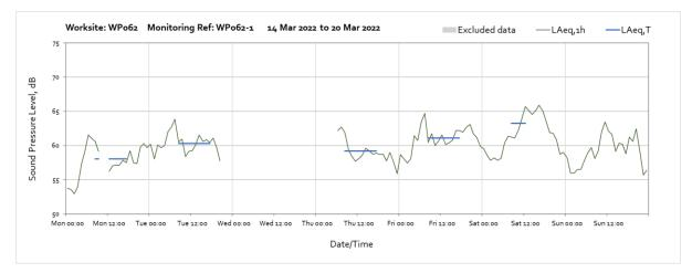
Note: Missing data on 14<sup>th</sup> March (10:00-11:00) and between 15<sup>th</sup> (21:00) to 17<sup>th</sup> March (06:00) was due to outage period for noise monitor 1.
