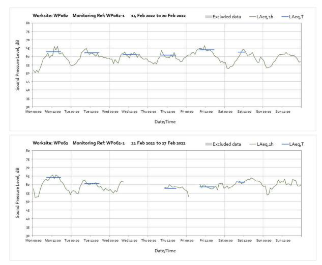
Note: Missing data between 09:00 on Wednesday 23<sup>rd</sup> February and 10:00 on Thursday 24<sup>th</sup> February was due to high winds knocking the solar panel over leading to loss of battery power. The equipment was repositioned on 24<sup>th</sup> February. Missing data between 02:00 and 08:00 on Friday 25<sup>th</sup> February was due to lack of battery charge, no works were being undertaken during this time.
