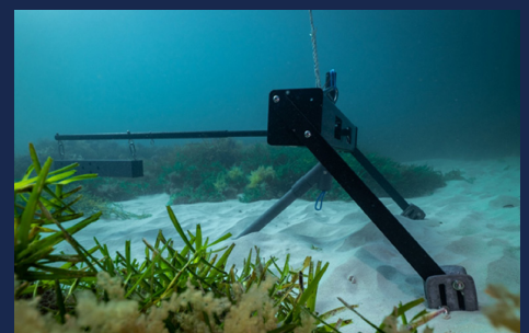
Baited Remote Underwater Video Systems, or BRUVS, in open ocean, ready to deploy on board, and in seabed habitats
