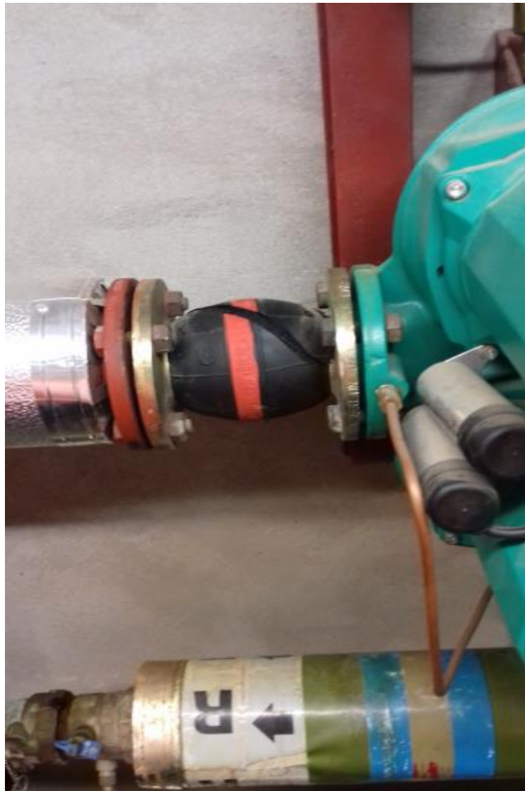
Photograph 1 failed and rubber split bellows seal
