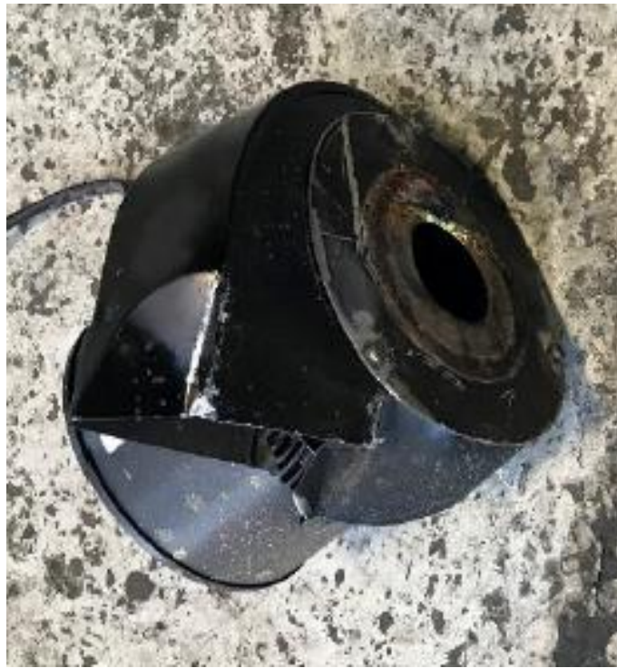
Photograph 1: Fan motor assembly with missing spigot that locates onto the radiator heat emitter tube pipe (see Photograph 3)
