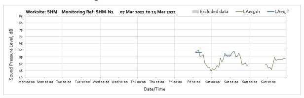
Note: Missing data from the beginning of the month till 11<sup>th</sup> of March and between 00:00 to 10:00 on 13<sup>th</sup> March were due to loss of power to the equipment as the solar panel fell-off the bracket because of the storm experience in the beginning of March.
