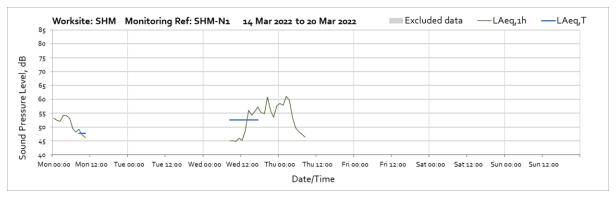
Note: Missing data from 11:00 on 14<sup>th</sup> March to 08:00 on 16<sup>th</sup> March and from 09:00 on 17<sup>th</sup> March till the end of the week was due to loss of power to the equipment as the solar panel fell-off the bracket because of the storm experience in the beginning of March.
