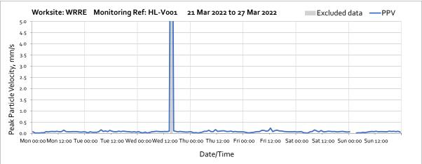
Note: High vibration levels measured at 15:00 on Wednesday 23<sup>rd</sup> March 2022 were due to local disturbance at the monitoring location and not representative of HS2 vibration levels at the receptor. Missing data in between 01:00 and 02:00 on Sunday 27<sup>th</sup> March was due to the clocks going forward at the start of British Summer Time.
